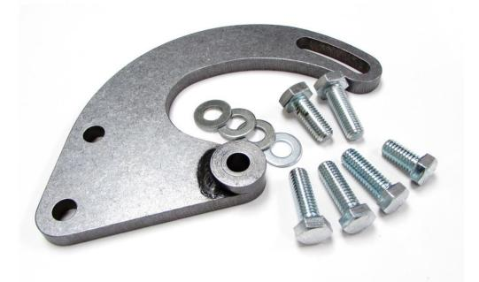
**\*\*Note**: Bracket is intended for use with Saginaw self-contained power steering pumps with two mounting locations on the back or the reservoir. Contains bolts for both metric and SAE threaded pumps.
