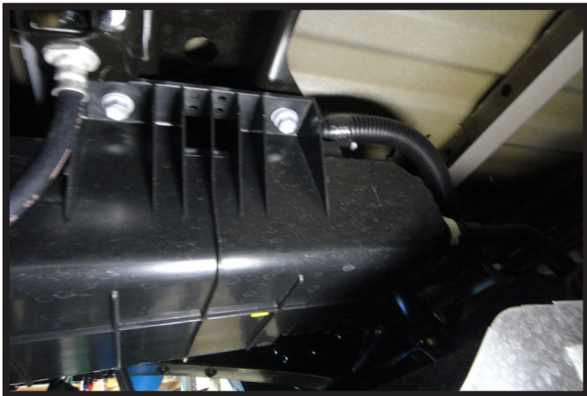
8. If equipped on newer models to ease installation, remove the evaporator canister temporarily. Once the center section is installed the canister can be reinstalled.
