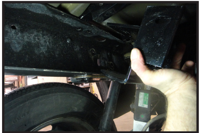
9. Install the frame bracket into the inside of the frame between the cross members. Do this on both sides of the vehicle. Do not fully tighten hardware at this time. Note: On the passenger side insure to straddle the wiring loom so that it sits inside the frame cavity.
