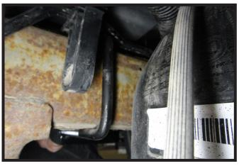
Install the u-bolts from the inside of the frame thru the side plates and install hardware. Do not fully tighten at this time. Do this on both sides of the vehicle.
