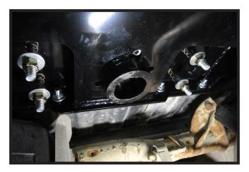
12. Using a 19/32" drill bit, drill the two (2) holes closest to the ball thru the bed. Do this on both sides of the center section.
