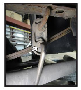
Drop the exhaust by sliding the rear hanger out of the rubber insulator.
