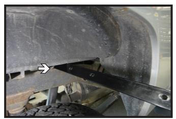
7. From the passenger side, slide the front cross member in from the side forward of the bed rail. Lift up on the angle to slightly bend the bed lip. Slide the cross member across the frame.
