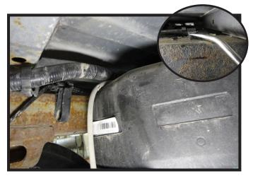
4. Remove the push pin from the wiring loom on the driver side and temporarily relocate the loom for cross member installation.
