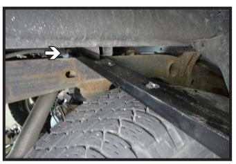
6. From the passenger side, slide the rear cross member in from the side just behind the bed rail. Slide the cross member across the frame, then flip the cross member upright. The center four (4) holes should be offset towards the bottom.
