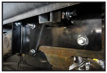
Install the side plates onto the cross members with the supplied hardware. Do this on both sides of the vehicle.
