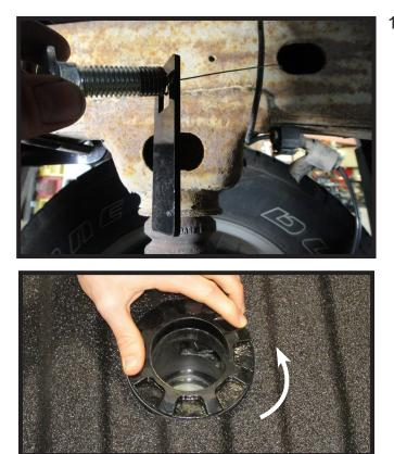
11. Install the fishwire into the large hole in the side plate thru the frame. Install the plate & carriage bolt onto the fishwire and pull thru the frame into the side plate. Install the lock nut onto the bolt. Do this on both sides of the vehicle.
