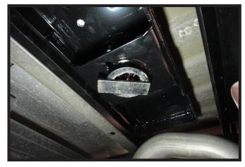
6. Install the center section up thru the 5" hole in the bed and in between the crossmembers. Being careful not to tear the tape when install the socket housing thru the bed hole and secure in place.
