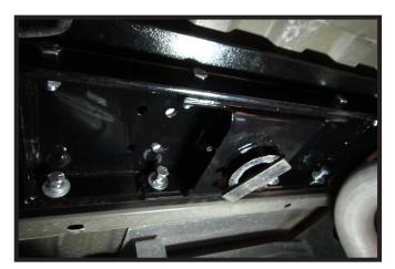
Secure the center section to the crossmembers with the appropriate hardware. Do not fully tighten the fasteners.
