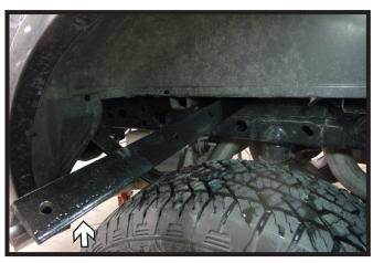
5. On the passenger side, slide the rear crossmember across the top of the frame just in front of the bed rail.
