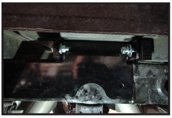
8. On both sides of the vehicle, bolt the side plates to the crossmembers using the appropriate hardware. Do not fully tighten hardware.
