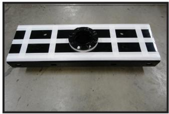
3. On the top side of the center section, apply the poly tape as shown to prevent galvanic corrosion. Insure the tape around the collar does nit interfere with it's function. (Tape shown in white for clarity)
