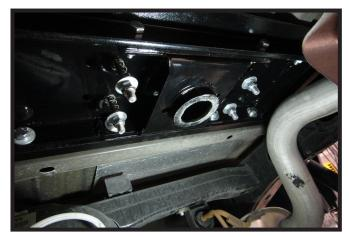
11. Using a 17/32" drill bit, drill the inner set of safety chain holes thru the bed. Do this on both sides.
