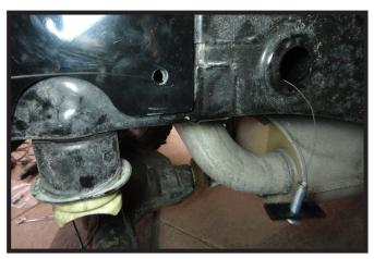
9. Install the fishwire into the sideplate hole and out thru the frame access hole. Place the locking plate and carriage bolt onto the fishwire and pull back thru the frame hole. Remove the fishwire and install the lock nut onto the bolt. Repeat for each frame hole. Do not fully tighten hardware.
