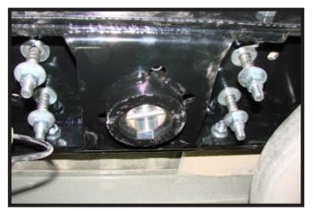
15. Insert the 1/2"-13 u-bolts thru the holes from the topside. Install a 1/2" flat washer, spring, another 1/2" flat washer and 1/2"-13 lock nut onto each u-bolt stud. Tighten until the washers are touching the spring without compressing it.
