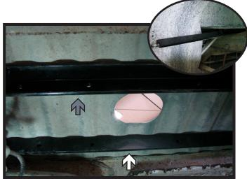
7. Slide each cross member in on top of the frame on the driver side just in front of the wheel well (inset).
