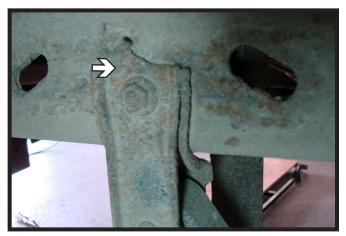
3. Using a 13MM socket, remove the bolt from the rear exhaust hanger.
