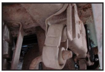
16. Reinstall the factory exhaust bracket. If the exhaust pipe sits too high and interferes with the hitch, cut the rubber hanger off of the exhaust bracket and install the supplied adjustable exhaust hanger Reinstall the spare tire per the vehicles owners manual.
