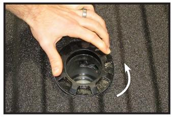
13. Check the rotation of the top collar at this time to insure the bed is not rubbing against it and it can rotate freely. If necessary drop the center section and remove any obstructions.
