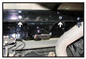
8. Install the center section, aligning it with the 5" hole in the bed.
