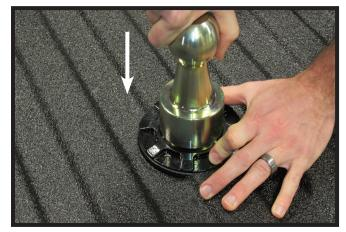
2. Align the ball with the collar and drop the ball into the hitch. Release the locking collar.
