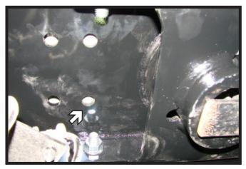
14. Using a 19/32" drill bit, drill the two (2) holes closest to the ball thru the bed. Do this on both sides.
