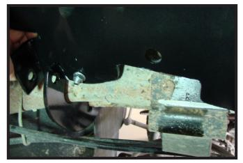
11. Slide the side plate in between the frame and the outer hook of the j-clamp, and position it into the studs of the crossmembers and the j-clamp. Do this on both sides of the vehicle.
