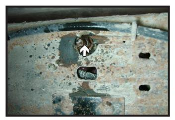
4. Using a 15MM socket, remove the nut from the emergency brake holder.
