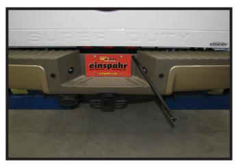
1. Using the vehicles jack handle tool, remove the spare tire as per vehicles owners manual.
