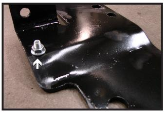
10. Install the 5/16" carriage bolt thru the square hole in the driver side plate only with the nut on the outside.
