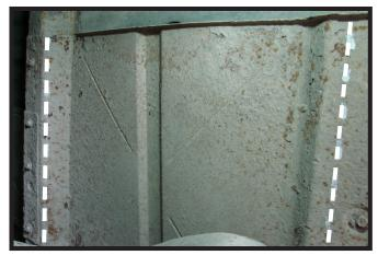
5. If equipped, trim and discard the exhaust heat shield in the area shown.
