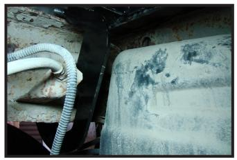
Position the J-clamp around the inside of the frame, next to the front cross-member. Do this on both sides of the vehicle.
