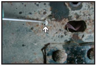
6. Locate the wiring loom clamp secured thru the hole in the driver side frame. Trim and push the clamp thru the frame.
