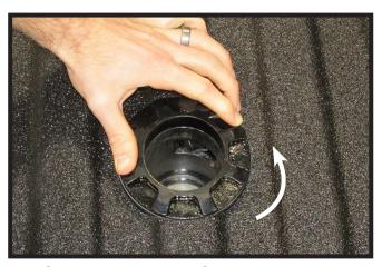
Check the rotation of the top collar at this time to insure the bed is not rubbing against it and it can rotate freely. If necessary drop the center section and remove any obstructions.
