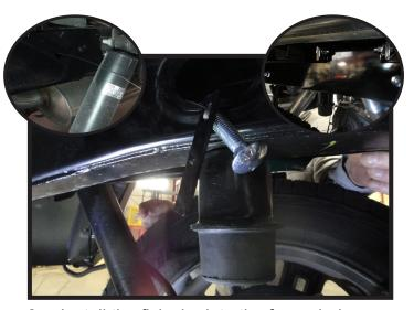
8. Install the fishwire into the frame holes and out the inner frame access hole. Place the locking plate and carriage bolt onto the fishwire and pull back thru the frame hole. Remove the fishwire and install the lock nut onto the bolt. Repeat for each frame hole.
