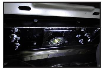
10. Using a 17/32" drill bit, drill the two (2) holes thru the bed that land in the bed valley. Do this on both sides.
