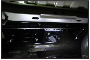
Secure in the center section to the crossmembers with the appropriate hardware. Do not fully tighten the fasteners.
