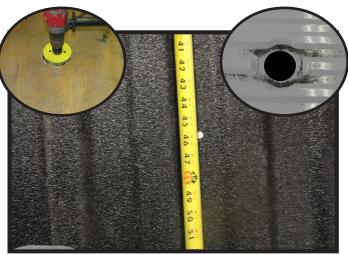
2. Measure and mark a hole at 45-3/4" from the end of the bed (not the tailgate) and centered between the wheel wells. Drill a 5" hole thru the bed. When a bed liner is installed, compensation of the bed liner thickness must be accounted for when measuring the ball location in the box bed.
