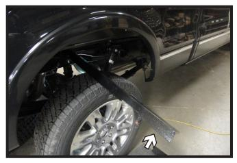
3. On the passenger side, slide the rear crossmember across the top of the frame towards the rear of the bed hole.
