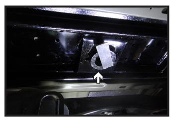
5. Install the center section up thru the 5" hole in the bed and in between the crossmembers.
