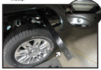
4. On the passenger side, slide the front crossmember across the top of the frame towards the front of the bed hole.
