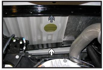
5. Install the rear cross member (36-1/2"L) in front of the hole then slide back to the backside of the hole (gray).
