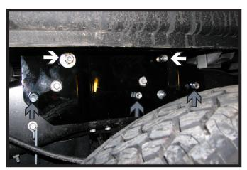
On the driver side, attach the support plate to the 5/8"-11 studs of the cross member with a 5/8" washer on the slotted end and 5/8"-11 lock nuts on both (white). Install 1/2"-13 x 1-1/2" bolts with 1/2"-13 lock nuts into the lower three (3) holes, with a 1/4" spacer on the inside of the middle hole (gray).
