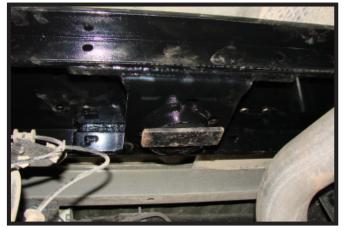
6. Install the center section, aligning with the hole in the bed. Secure in place.
