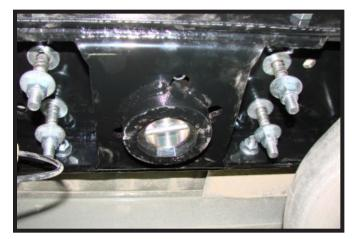
Fully tighten all cross member/center section hardware. Then using a 19/32" drill bit, drill the two (2) holes closest to the ball thru the bed. Do this on both sides.
