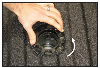
10. Check the rotation of the top collar at this time to insure the bed is not rubbing against it and it can rotate freely. If necessary drop the center section and remove any obstructions.
