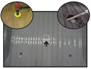
2. On the inside of the bed, measure from the rear (not the tailgate) forward 46-1/8" and mark. Measure between the wheel wells and mark center. Using a 5" hole saw, drill a hole thru the bed.
