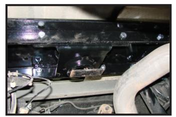
On both sides of the center section, bolt the cross members to the center section with four (4) 1/2"-13 x 1-1/2" bolts with 1/2" washers and 1/2"-13 lock nuts on the inside. Do not fully tighten hardware.
