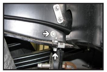
On the passenger side only, using a 10MM socket, remove the two (2) bolts from the exhaust hanger.
