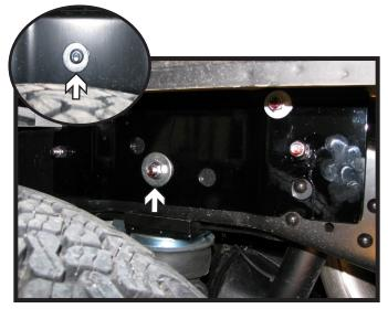
9. Repeat the same steps from step #8 on the passenger side. If the vehicle is equipped with air bags, the nut and washer must be removed prior to support plate installment (inset). Then reattach the washer and nut to the stud after the support plate is installed. Fully tighten both support plates hardware.
