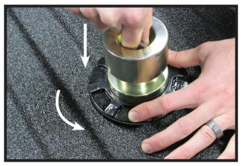
1. Rotate the locking collar to release the latch pawl. Align the ball with the collar and drop the ball into the hitch.
