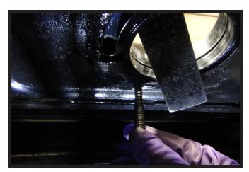
11. Ensure the drilled holes are centered with the tapped holes in the top assembly.
