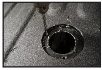
6. Using a 3/8" drill bit, bore out the previously drilled pilot holes.
