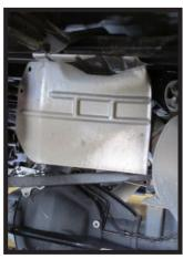
3. Using a 10MM socket, remove the four (4) bolts from the heat shielding. There are two (2) toward the top of the shielding, and two (2) toward the bottom. Bend the shielding away, as shown.
