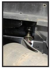
10. Insert the nut plates in the wheel well between the box and frame, and insure the plates are centered. Do this for both sides of the vehicle.
