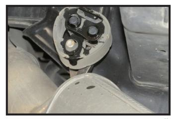
4. Drop the exhaust by sliding the hanger off the rubber insulator.
