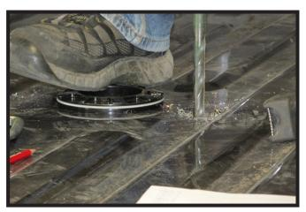
13. Using the safety chain template, mark and drill pilot holes from on top of the truck bed.
