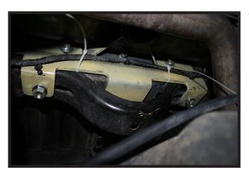
11. Reattach the wiring harness by using the cable ties that were provided.
