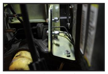
10. Place the support plate onto the frame side. Install the 5-1/2" x 4-1/4" u-bolt and finger tighten the nuts. Align top holes and install a 1/2"-13 x 1-1/2" bolt, 1/2" flat washer & lock nut. Do this on both sides of the vehicle. Do not tighten bolts at this time.
