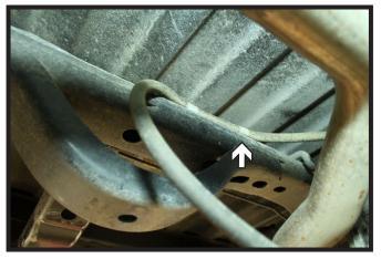
Unclip the vent tube and let it hang loosely. The vent tube will be relocated after the hitch is installed.
