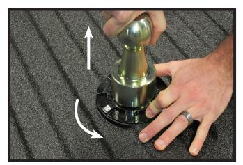
Rotate the locking collar to release the latch pawl. Pull straight up on the ball to remove from the hitch.
