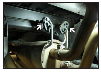
Drop the exhaust by sliding the hangers out of the rubber insulators.
