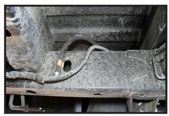
12. Looking towards the front of the vehicle, place the vent tube between the frame and brakes lines. Bring it up over the frame rail and clip it to the frame.
