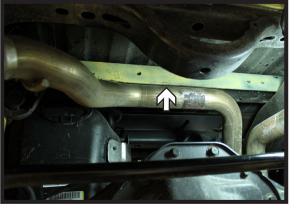
6. Slide the front angle up above the exhaust, between the frame and upper suspension. Rest it on the top of the frame until the cross member is installed. On the other side, slide the back support flat and rest it on the chassis frame. The notch on the back support flat should be facing toward the rear of the vehicle.
