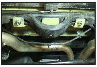
9. Attach the back support plate to the inside of the cross member. Insert the 1/2"-13 x 2" hex head bolts thru the back support plate and the threaded holes of the back support flat. Using the 5" bolt plates, reach through the frame and fasten the bottom of the back support plate. Tighten the bolts, the handle on the bolt plate will prevent the bolt from becoming loose.
