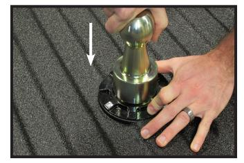
Align the ball with the collar and drop the ball into the hitch. Release the locking collar. Pull up on the ball to insure it is locked into the housing.
