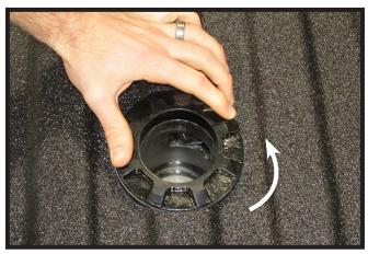
14. Check the rotation of the top collar at this time to insure the bed is not rubbing against it and it can rotate freely. If necessary drop the center section and remove any obstructions.
