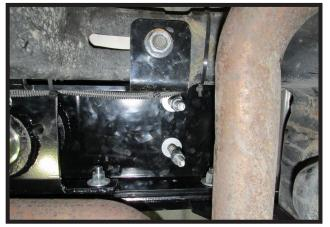
15. Using a 19/32" drill bit, drill the two (2) holes closest to the ball thru the bed. Do this on both sides of the center section. Insert the 1/2"-13 u-bolts thru the holes from the topside. Install a 1/2" flat washer, a spring, another 1/2" flat washer and 1/2"-13 lock nut onto each u-bolt stud. Tighten until the washers are touching the spring without compressing it.
