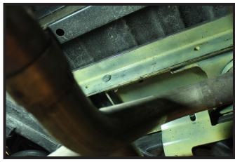
8. On the front angle insert the 1/2"-13 x 1-1/2" hex head bolts and nuts thru the center two (2) holes only. Insert the outer two (2) and center 1/2"-13 x 2" hex head bolts on the back support flat at this time also. Do not fully tighten at this time.
