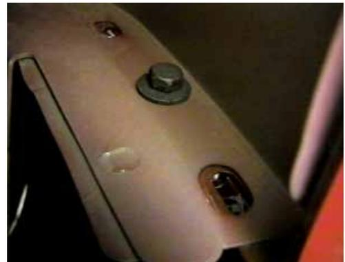
4. Using the 10MM socket, remove two metric bolts on fascia corner inside wheel well, both sides.
