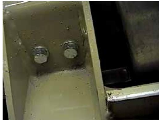
7. Hold baseplate to align with existing holes on frame (arrow shown in photo). Insert item 2 into frame opening, and fasten items 3, 4, and 5, both sides. Be sure baseplate is up as far as possible and drill remaining holes in frame rail with the 13/32" drill bit. Install items 2, 3, and 4 according to drawing on last page, tighten all bolts. **Be sure and loctite all bolts before tightening.**
