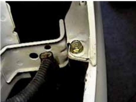
3. Just under headlight assembly, remove one push pin on fascia, both sides. Remove one metric bolt behind assembly with the 10MM socket, both sides.
