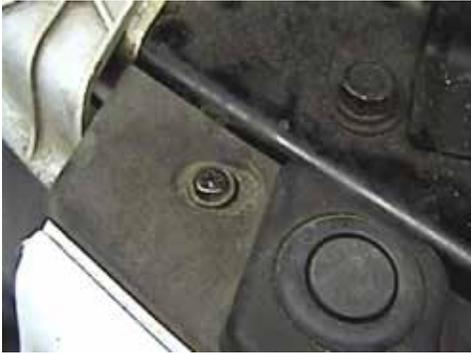
1. Remove the six push pins and six phillips head screws from black plastic on the top side of fascia and set aside.
