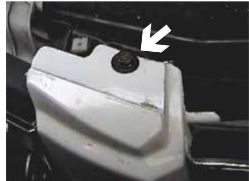
4. Remove two metric bolts from top side of fascia with the 10MM socket.
