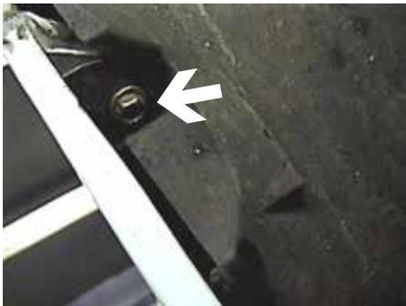
5. Using the 8MM socket, remove one metric bolt from upper fascia corner, just forward of front tires, both sides.
