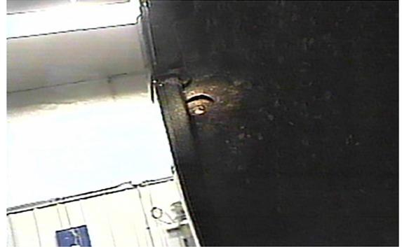
2. Use a 7MM socket to remove the three metric screws just forward of front tire wheel well, both sides. Remove eight push pins from bottom of fascia.
