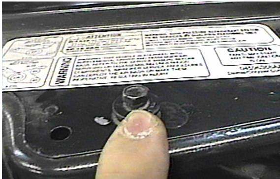
3. Remove the two metric bolts on the top side of the grill with 10MM socket. Pull fascia forward and set aside.
