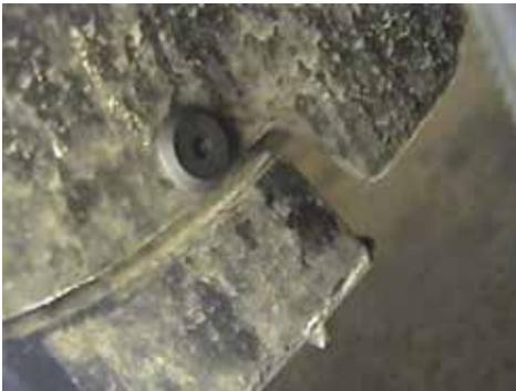
3. Just forward of front tires in wheel well, cut two pop rivets with the side cutters, both sides.
