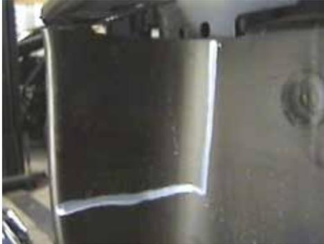
7. Measure 3" down from top of air dam and cut corner out to relieve area for baseplate, both sides.
