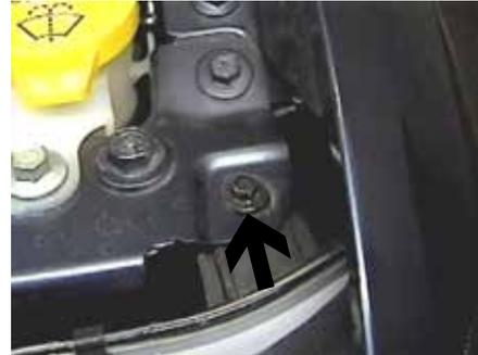
2. Using the 7MM socket, remove two metric bolts from the top of head light assembly, pull forward, both sides, and set aside.
