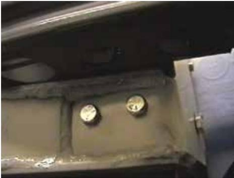
9. Drill remaining lower holes with the 13/32" drill bit, both sides. Insert items 2 into all drilled holes on baseplate, tighten items 3 and 4. **Be sure and use loctite on all bolts before tightening.**
