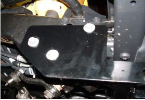
2. Hold baseplate (item 1) into place and insert the three existing bolts on passenger's side through baseplate, frame and gear box, tighten. Be sure and use Loctite on all bolts before tightening.
