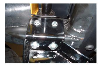
3. Clamp baseplate on driver's side with large vise grip and drill four holes with 13/32" drill bit.
