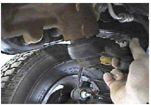
1. Remove the three metric bolts with 16MM socket while having someone hold the gear box and the idler arm.
