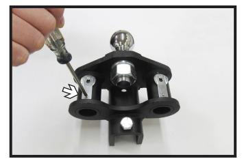
2. Using a Phillips screw driver, remove the screws at the bottom of the spring clip. Do this on both sides of the hitch head.
