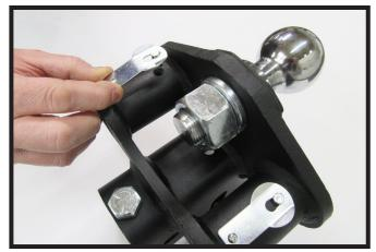
3. Remove spring clip and locking pin from the hitch head. Do this on both sides of the hitch head.
