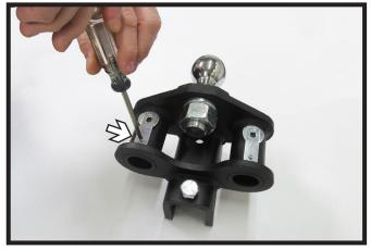
5. Apply Loctite<sup>®</sup> Red to the provided 6MM head screw and install in the bottom hole of the spring clip. Do this on both sides. Reinstall hitch head.
