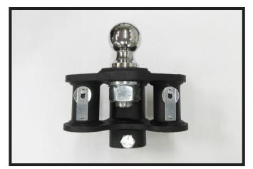
1. Remove hitch head from 2-Point system and set on a solid surface with springs facing upward.
