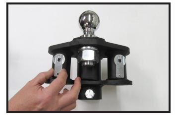
4. Place provided new spring clip and locking pin onto hitch head. Do this on both sides.
