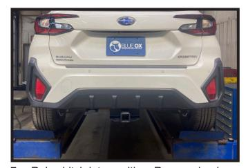
Raise hitch into position. Remove lead wires and loosely install 1/2" whiz flange nut onto each bolt. Then tighten all bolts.
