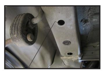
3. Feed wire through frame from rear hole to forward hole. Slide spacer plate onto 1/2" bolt and attach lead wire to end of bolt. Do this on both sides of the vehicle.
