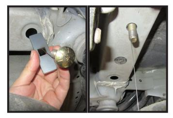
4. Pull bolt and spacer plate through forward hole to rear hole. Do this on both sides of the vehicle.
