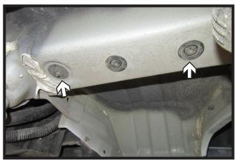
1. Remove the two (2) rubber plugs from the frame rail. Do this on both sides of the vehicle.
