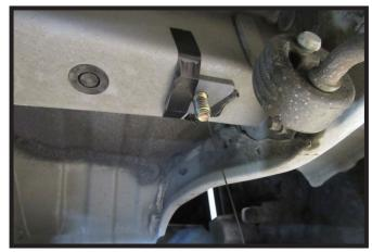
6. Do not remove lead wire. Hold receiver hitch up to frame. Determine if the 1-1/2" x 2" x 1/4" is needed to level hitch. If needed, tape spacer plate to frame as shown. Do this on both sides of the vehicle.
