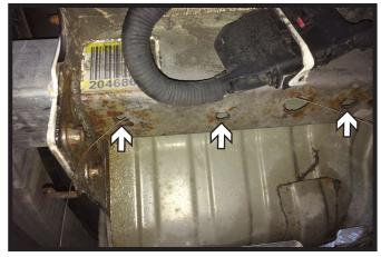
Feed a lead wire from the three (3) bolt holes in the frame to the access hole.
