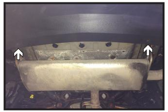
1. Using a T15 Torx, remove the two (2) bolts from the rear bumper.
