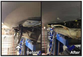
4. Remove rubber piece from rear exhaust hanger. Do this on both sides of the vehicle.
