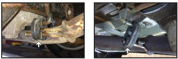
2. Support the exhaust and remove the two (2) rubber isolators from exhaust rods.
