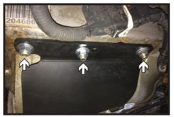
8. Raise hitch into position. Remove lead wires and loosely install a 1/2" whiz flange nut onto each bolt. Do this on both sides of the vehicle. Then tighten all bolts.
