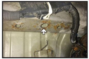
5. Using a rotary tool, grind out the access hole in the frame to 1-1/4". Do this on both sides of the vehicle.
