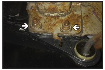
Using a 15MM socket, remove the two (2) bolts from the rear side of the frame bracket. Do this on both sides of the vehicle. Lower exhaust to allow clearance for receiver hitch installation.
