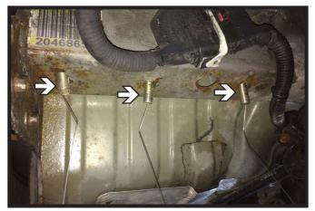
7. Pull bolts through the frame. Ensure the spacer plates are sitting flush against the inner frame and the bolts are hanging vertically. Do this on both sides of the vehicle.
