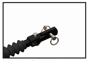
2. Install the offset double lug onto the tow bar leg with the new washers, 1/2"-13 bolt and 1/2"-13 jam nut provided. Tighten the bolt until the lug is tight against the washers, but can still freely move side to side. Do this on both tow bar legs. Note: Two different 1/2"-13 bolts are provided, use the correct bolt for the corresponding tow bar.
