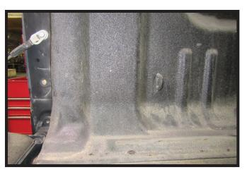
4. Locate a convenient mounting point (usually on the driver's side between the rear post and the wheel well area) and route the harness to this location.
