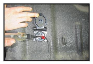
Confirm harness operation with a test light or by using a properly equipped trailer. Secure the extension harness cable to the vehicle using the cable ties provided.
