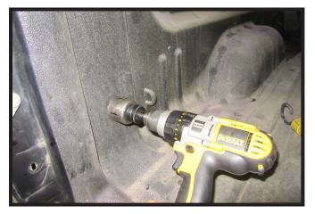
5. Using a hole saw, drill a 2-1/8" hole in the desired location in the sidewall. With a file, smooth the edges of the hole for a better fit of the harness and connector.
