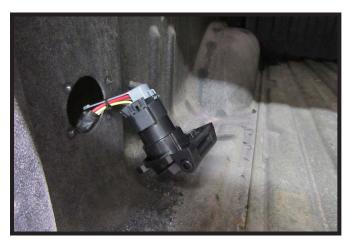
Route the extension harness connector up from under the body through the hole drilled in step 5. Insert the harness connector into the rear of the provided 7-way socket, pressing together to fully engage the locking tab.
