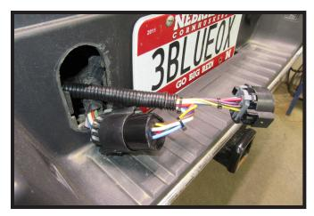
3. Attach provided harness into the vehicle's wiring harness connector, and into the rear of the factory 7-way socket. Insert fully to engage the locking tab. Return the locking clip to original position.
