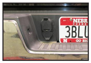
Locate the factory OEM trailer light wiring harness on the underside of the vehicle. The wiring harness will be connected to the vehicle's 7-way trailer connector which is mounted to the hitch or bumper at the rear of the vehicle. The vehicle harness will have a similar connector with a mating fit to one of the connectors on the 5th wheel harness.
