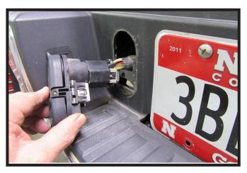
Disconnect the 7-way connector from the vehicle wiring harness by carefully releasing the locking clip and gently pulling the connector apart while holding down on the connector locking latch.
