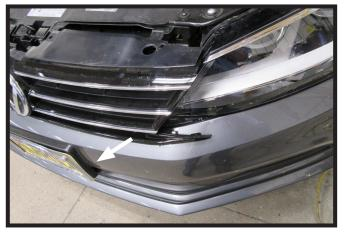
Release the clip on the lower part of the grille on both sides of the vehicle, pulling forward to release it and set the grille aside.
