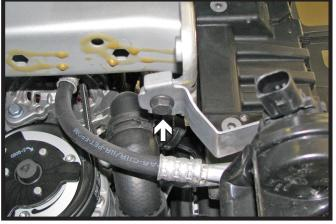
12. Using the 13MM socket, remove the bolt from the horn bracket. Unplug the electrical connection and set the horn assembly aside. Do this on both sides of the vehicle.
