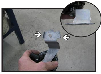
20. Flatten the horn bracket tabs on the passenger side only. Reinstall both horn brackets and plug in the electrical connections.
