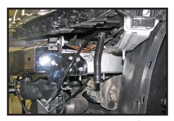
24. Attach the permanent baseplate safety cables to the provided convenience link on the baseplate. The photo above shows the recommended installation of the cables to frame of vehicle. Additional options may interfere with suggested mounting; in this case, secure the cables to a solid piece of the frame as described in the General Information sheet. Be sure the safety cables do not rub against any hoses or moving parts. Do this on BOTH sides of the vehicle.
