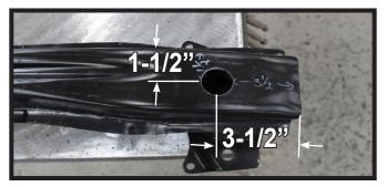
17. On the passenger side, enlarge the hole on the front of the metal bumper just forward of the center of the frame end. Use a reciprocating saw and enlarge the hole or drill out with an 1-1-4" hole saw.
