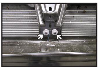
9. Using a 10MM socket, remove the two (2) nuts from the middle of the bumper and set the bumper aside.
