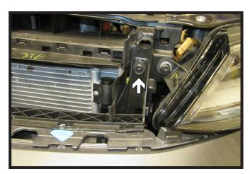
3. Using the T30 Torx, remove the two (2) screws from the fascia. There is one (1) on each side.
