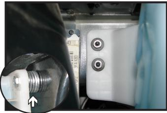
21. Put the washer reservoir in place on the back two studs and loosely reinstall the two (2) hex nuts. Use the 6MM hex bolt provided on the front hole with flat washers as spacers to prevent webbing from rubbing a hole in the reservoir tank. Tighten the back nuts and reconnect all the electrical and fluid lines to the reservoir.
