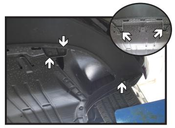
5. Using a 25 Torx, remove the eight (8) screws from the underside of the fascia. There are three (3) on each corner and two (2) in the center.
