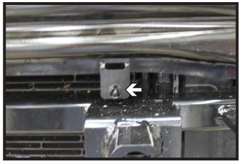
19. Drill a 1/2" hole in the plate as shown above and insert temperature sensor into hole
