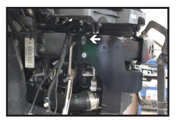
18. Slide the baseplate into position, centering the slot in the baseplate horizontally with the existing hole in the frame. Flush the baseplate with top of the frame. Level and clamp the baseplate into position.
