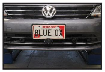
25. Reinstall the stryofoam bumper. Hold the fascia as close to its original position, mark and trim the fascia around the convenience links and attachment tabs. Reinstall the fascia.
