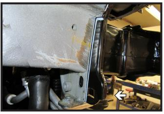
14. Temporarily reinstall the metal bumper. Mark the back side of the bumper along the frame cut out. Do this on both sides. Remove the bumper, then cut out the areas with a reciprocating saw. Then reinstall the bumper fully tightening all fasteners.
