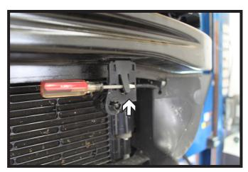
7. Unplug and remove the temperature sensor (white arrow). Take the center piece off for now.
