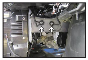
11. On the driver side, using a 10MM socket remove the two (2) nuts holding the ground wires. Move the ground wires out of the way. Cut the studs flush with the frame rail.
