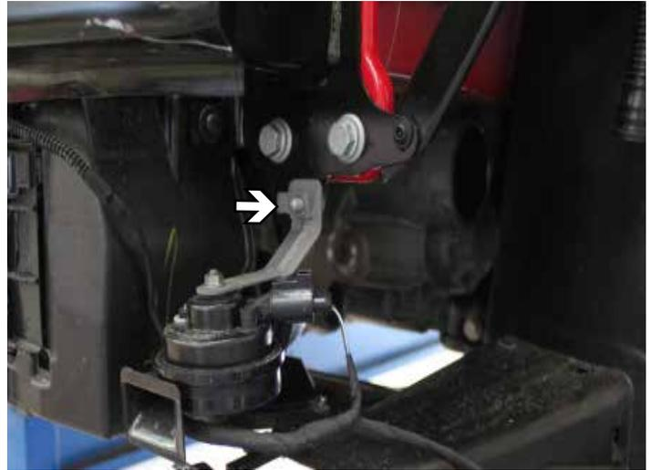
10. Using a 50 Torx, remove the one (1) screw at the top of the horn bracket, unhook the wiring and set aside. Repeat on other side.
