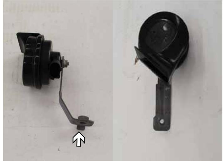
14. Flatten out the horn bracket with a hammer on a solid surface. Then remove the side tab with pliers or vise-grips by twisting back & forth (shown above to left). Bracket should look like right hand picture when done. Repeat on other horn.
