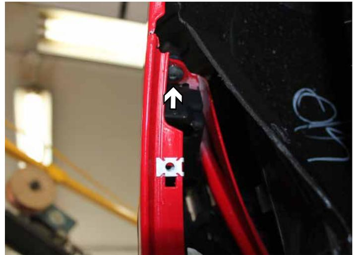
4. Behind the wheel well cover remove the one (1) upper fascia screw with a 25 Torx. Do this to both sides of the vehicle.
