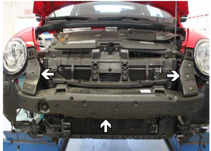
8. Remove the three (3) foam fascia support pieces. DO NOT discard these will be reinstalled.
