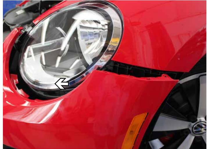
6. When removing front fascia, pull straight out and unhook both the side marker and running light wiring on both sides of vehicle.
