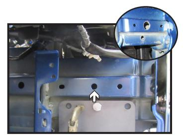
Using a 1-1/4" drill bit ream out the existing hole to 1-1/4" to create an access hole. Do this on both sides of the vehicle.
