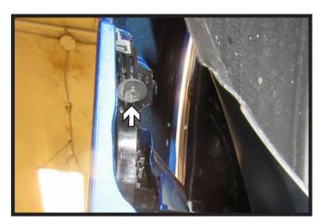
Pull back the wheel well cover, the using an 8MM socket remove the one (1) bolt. Do this on both sides of the vehicle.
