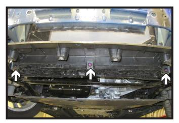
Using a 10MM socket remove the three
