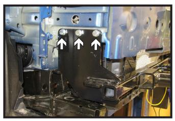
14. Insert three (3) 3/8" bolts with lock washer and whiz nuts into the side plate of the baseplate. Do this on both sides of the vehicle.
