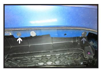
6. Pull down the belly pan, then using an 8MM socket remove the one (1) bolt (white) and one (1) push pin (gray). Do this on both sides of the vehicle.
