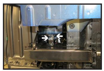
12. Attach the baseplate to the bracket using two (2) 3/8" bolts with lock washer and nylon lock nut. Do this on both sides of the vehicle. Tighten all bolts fully at this time.
