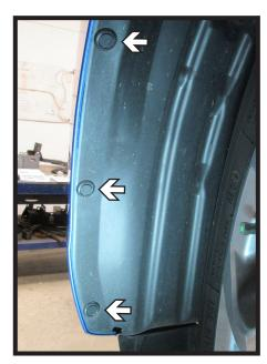
3. Remove the three (3) push pins in front of the tire in the wheel well. Do this on both sides of the vehicle.
