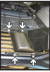
18. Using a Phillips screw driver remove the six (6) screws attaching the two (2) plastic pieces to the back side of the fascia. There are four (4) screws on the driver side and two (2) on the passenger side. Once the pieces are removed reinstall all screws.
