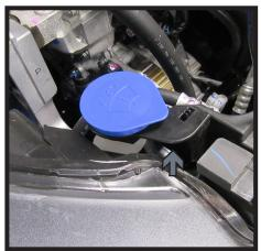
7. Using a 10MM socket remove the three (3) bolts (white) from the windshield washer reservoir. Then pinch together the black piece (gray arrow) holding the blue reservoir cap, to remove from the frame. Unplug all lines, remove the reservoir, and set aside to be reinstalled later.
