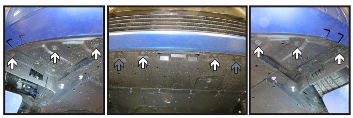
5. Using an 8MM socket remove the eight (8) bolts (white) from the under side of the fascia. Then remove the two (2) push pins (gray).
