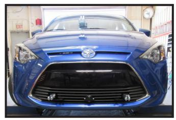
19. Hold the fascia as close to its original position, mark and trim the fascia around the convenience links and attachment tabs. Reinstall the fascia and fascia cover.
