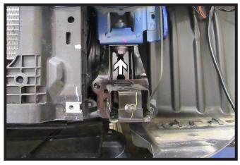
Using a 17MM socket with extension remove the one (1) bolt coming from the underside. Do this on both sides of the vehicle.
