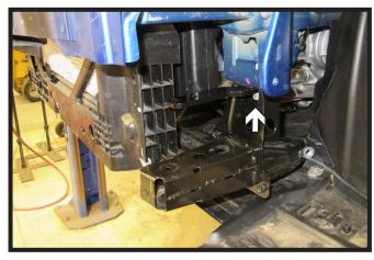
11. Use the existing 12MM bolt attach the bracket to the frame, leave loose. Do this on both sides of the vehicle.
