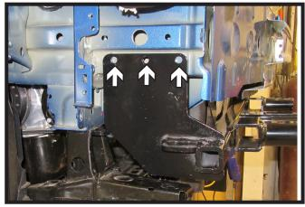
13. Using a 3/8" drill bit, drill the top three (3) holes for the baseplate. Do this on both sides of the vehicle.
