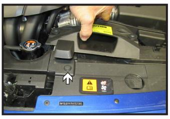
Lift up the plastic piece on the driver side of the vehicle and remove the one (1) push pin.
