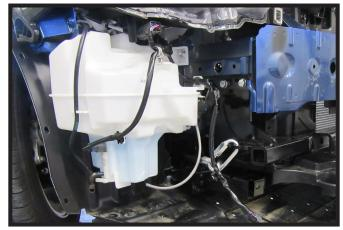
17. Reinstall the windshield washer fluid reservoir on the passenger side of the vehicle.
