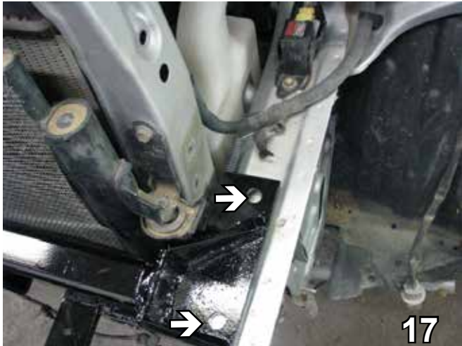
17. Continuing on the driver's side, drill the two holes with the 17/32" drill bit using the baseplate as a template.
