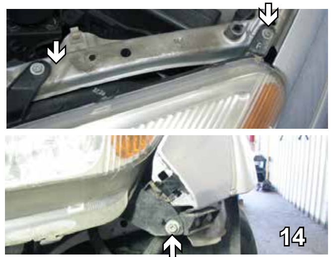
14. Use a 10MM socket to remove the three bolts from the headlight assembly, two on the top and one on the bottom. Pull out the assembly in order to drill the holes but do not disconnect the wiring.
