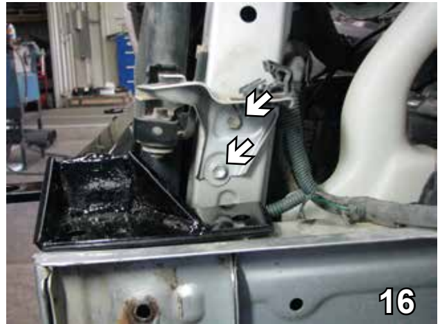
16. On the driver's side, use a 10MM socket to remove the two bolts from the brace.
