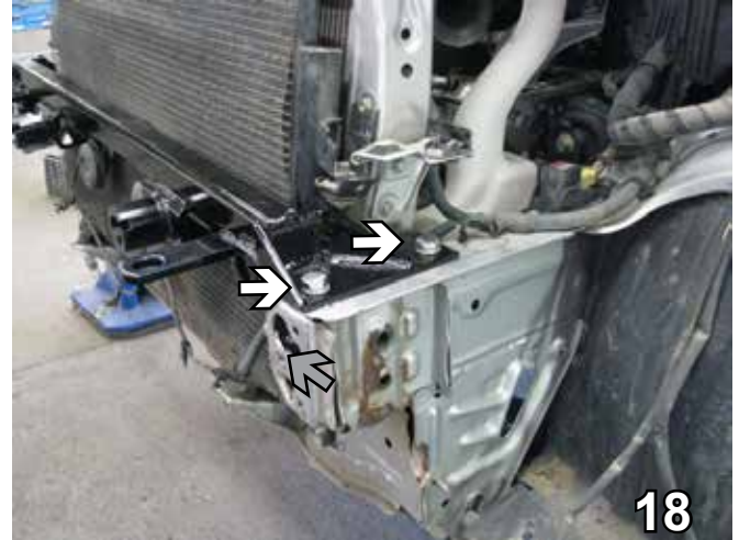
18. Install 1 1/4" bolts with 1/2" lock washers into the drilled holes, tighten with 1/2" nut plates inserted into the hole on the side (gray arrow). Be sure to use Loctite Red on all bolts. Do this on both sides, driver's side shown.
