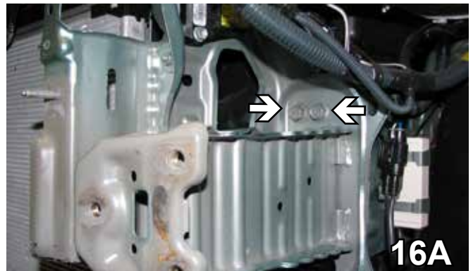
14. Line up the two big existing holes in the frame extension with the side baseplate holes. Start the 3/8-16 x 1 1/4" bolts with 3/8" lock washers and on the inside of the frame use 3/8-16 nut plate. Do this on both sides.
