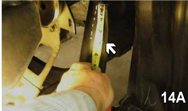
14. Below the frame, cut the plastic 3" down and 1 3/4" across.
