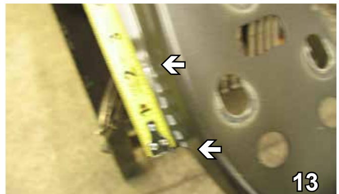
13. On the bottom side of the bumper, using a reciprocating saw trim back 2". Do this on both sides.
