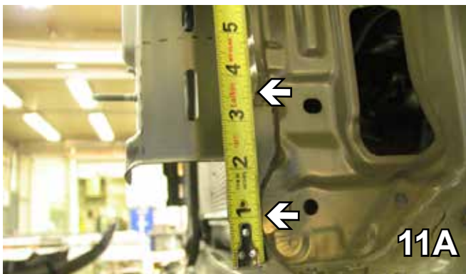
11. Using a reciprocating saw, cut a notch starting 1" up from the bottom and continuing 3 1/2" up (11A) in the lower frame support webbing and cut it out. Also cut out the area enclosed in the oval in 11B. Do this on both sides.
