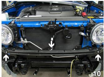
10. Using the 10MM socket, remove three bolts from the fascia support crossbar. Pull the crossbar forward to remove. Set bolts and crossbar aside to be reinstalled later.
