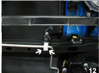
12. On the driver's side, squeeze the back side of the plastic retainer clip holding the coolant tubing. Pull retainer clip forward to release the coolant tubing from the bracket.
