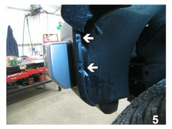
5. Using the 10MM socket, remove two metric bolts from the outside edge of wheel well, just forward of the front tire. Do this to both sides of the vehicle. Set bolts aside to be reinstalled later.
