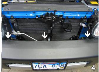
4. Remove three push pins just behind the top edge of the bumper. Set push pins aside to be reinstalled later.
