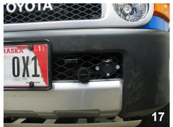
17. Reinstall the belly pan, grille, metal bumper, and fascia support crossbar. Hold the fascia up to its original location. Mark and trim the grille with the utility knife as necessary for the attachment tabs, convenience links, and electrical rods. Reinstall the fascia.
