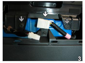
Disconnect the electrical connection (see white arrow). Remove two Phillips screws (see grey arrows). Set screws aside to be reinstalled later.
