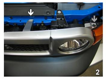
2. Using a 10MM socket or Phillips screwdriver, remove the hex bolt from the grille support bracket (see white arrow). Remove the pushpin from the upper, outside edge of grille assembly (see grey arrow). Do this to both sides of the vehicle. Set bolts and push pins aside to be reinstalled later.
