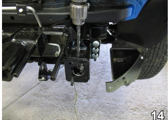
14. With the baseplate on top of the frame rail extension, use the baseplate as a template to drill two holes in the top of the extension with the 13/32" drill bit. Insert 3/8" nut plates into frame rail extension and align with drilled holes. Install 3/8-16 x 1 1/4" bolts and 3/8" lock washers to the baseplate and tighten to nut plates using the 9/16" socket. Trim nut plate wires. Do this to both sides of the vehicle.
