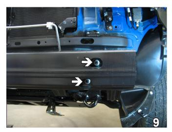
9. Using the 14MM socket, remove two metric bolts from the metal bumper. Do this to both sides of the vehicle. Pull metal bumper forward to remove. Set bolts and bumper aside to be reinstalled later.
