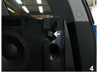
4. Remove one Phillips screw from each of the upper corners of the subwoofer case. Remove the subwoofer. Set screws and subwoofer aside to be reinstalled later.
