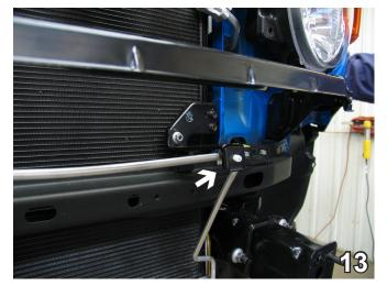
13. Slide the coolant tube behind the bracket. Rotate the retainer clip and insert into the back side of original bracket location to open the area for baseplate installation.
