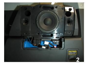
2. Use a flat screwdriver to pry upward on the panel below subwoofer to remove it. Or, pull forward on upper part of panel. Photo shows panel removed.
