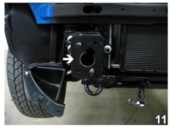
11. Using the 1 1/4" hole saw, drill out the center of the frame rail end plate. *Note: The cut should overlap the existing hole*. Do this to both sides of the vehicle.
