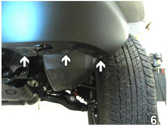
6. Using the 10MM socket, remove three metric bolts from the bottom corner of fascia, just forward of the front tire. Do this to both sides of the vehicle. Set bolts aside to be reinstalled later.
