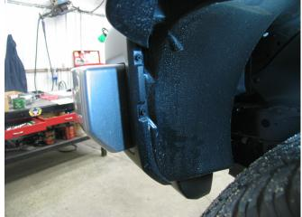
8. Grasp the top edge of the fascia's corner, just forward of the front tire and carefully push the fascia's corner towards the front tire, then pull to the side to release fascia. Do this to both sides of the vehicle. Pull fascia forward to remove. Set fascia aside carefully to be reinstalled later.
