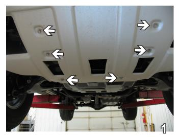
1. Using the 12MM socket, remove six metric bolts from the belly pan. Set belly pan and bolts aside to be reinstalled later.
