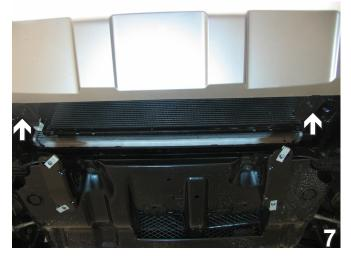
7. Using the 10MM socket, remove two metric bolts from the bottom edge of the fascia, just forward of the radiator. Set bolts aside to be reinstalled later.
