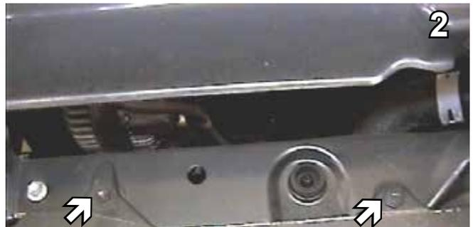
2. Remove two metric bolts from top edge of fascia's tabs with the 10MM socket. Remove one push pin.
