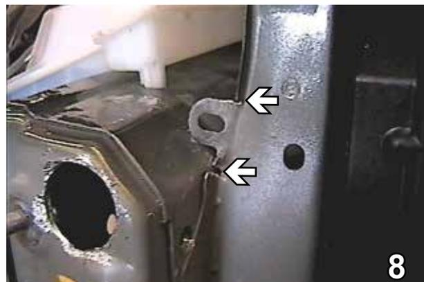
**Using a good quality paint, spray cut edges of frame to prevent rusting.**
