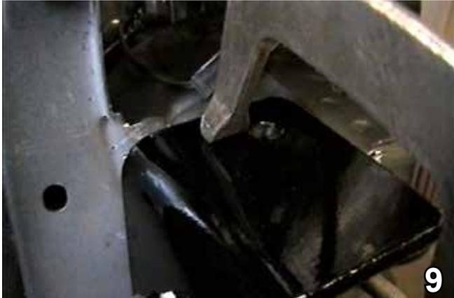
9. Set baseplate on top of frame ends and clamp in place. Baseplate should be firm against the front of radiator support. Using the baseplate as a template drill three holes with the 13/32" drill bit, both sides.
