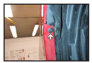
2. Remove the one (1) push pin from along the edge of the wheel well by pressing down on the center to release. Do this on both sides of the vehicle.
