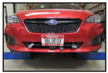
12. Hold the fascia as close to its original position, mark and trim the fascia around the convenience links and attachment tabs. Reinstall the fascia.
