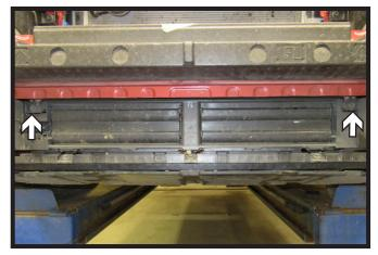
4. Using a 10MM socket remove the two (2) bolts attaching the bumper to the shutters.
