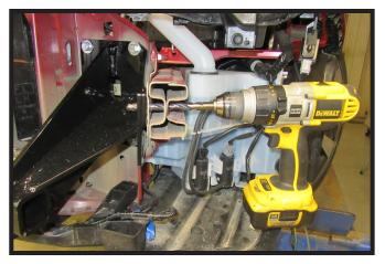
Using a 1/2" drill bit, drill a hole through the frame as indicated so that it meets up with the corresponding slotted hole on the baseplate. Do this on both sides of the vehicle.
