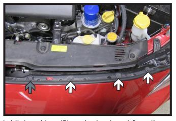
1. Using a 10 MM Socket remove the six (6) bolts (white) and two (2) push pins (gray) from the top of the fascia.
