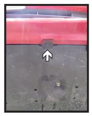
3. Remove the ten (10) push pins from the underside of the vehicle, five (5) on each side. Then remove the fascia and set aside to be reinstalled later
