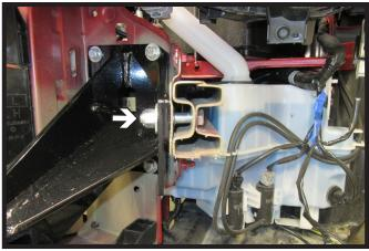
9. Install one (1) 1/2" x 2-1/2" bolt with flat washer and nylon lock nut. Do this on both sides of the vehicle.
