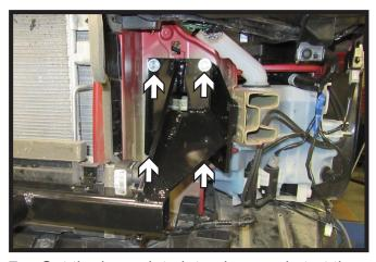
7. Set the baseplate into place and start the four (4) 8MM bolts with hardware. Do this on both sides of the vehicle. After all bolts have been inserted tighten fully.
