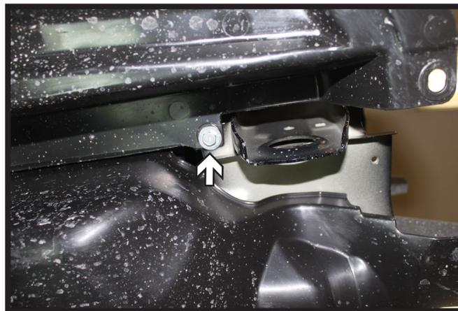
6. Using a 10MM socket, remove the bolt on the underside of the outer plastic shielding, letting the shield hang loose. Do this on both sides of the vehicle.
