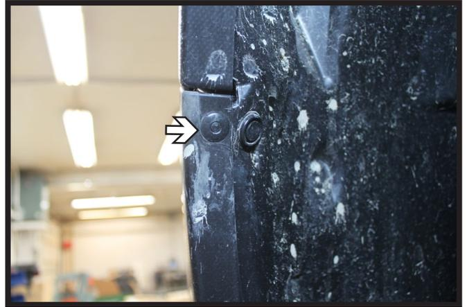
2. Release the pin from the top edge of the fascia/wheel well joint by pushing in on the center section. Do this on both sides of the vehicle.
