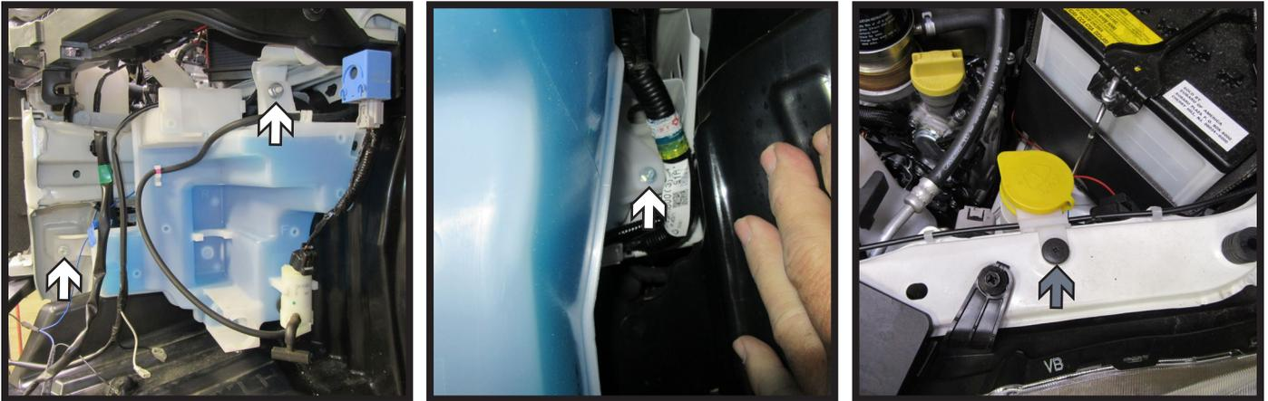
6. Using a 10MM socket, remove the three (3) bolts (white) from the washer reservoir. There is one (1) in front, one (1) at the top and one (1) behind the wheel well liner. Remove the Phillips push pin (gray) from the reservoir neck. Disconnect and plug all lines. Set the reservoir aside to be reinstalled later.
