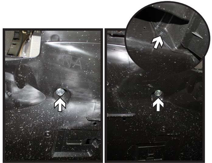
10. Using a 12MM socket, remove the two (2) screws from the underneath. Then remove the two (2) push pins from each side (inset). Drop the front of belly pan down for baseplate installation.
