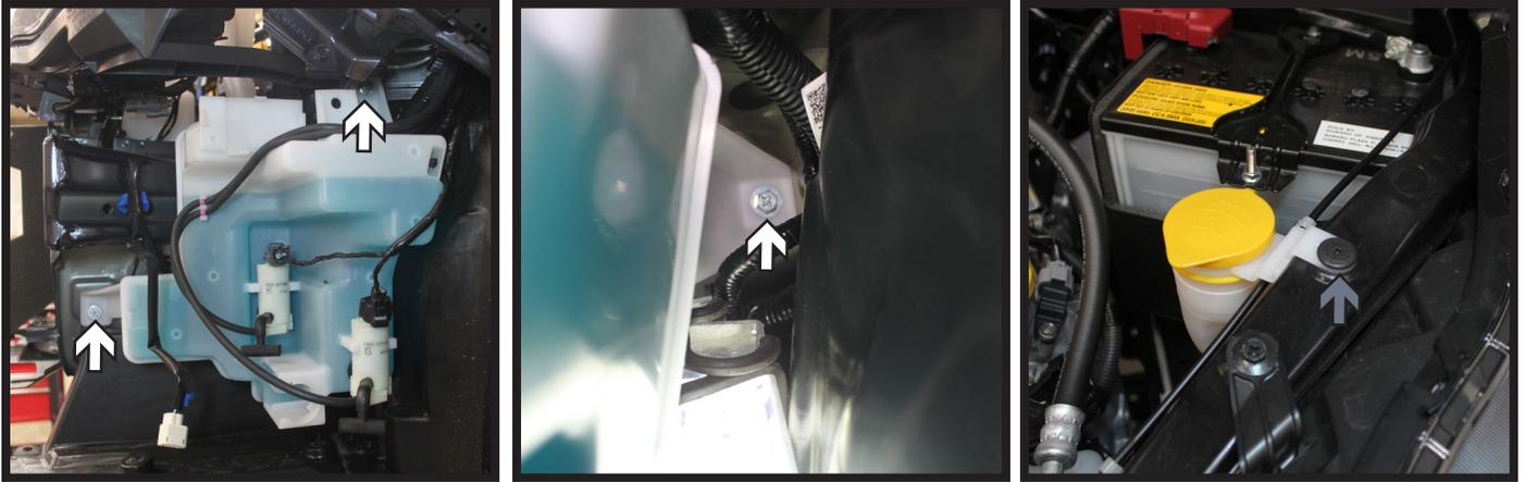
7. Using a 10MM socket, remove the three (3) bolts (white) from the washer reservoir. There is one (1) in front, one (1) at the top and one (1) behind the wheel well liner. Remove the Phillips push pin (gray) from the reservoir neck. Disconnect and plug all lines. Set the reservoir aside to be reinstalled later.
