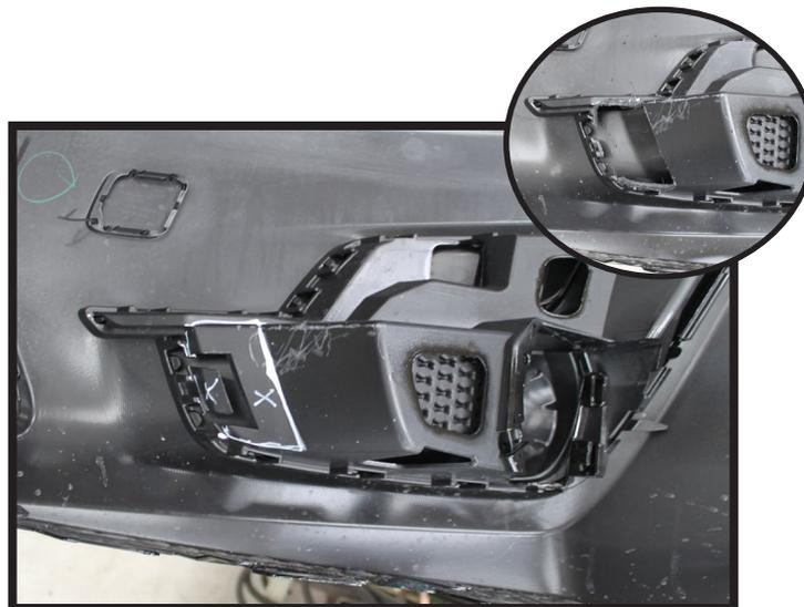
22. **Impreza:** Trim the indicated area on the back of the fascia to allow baseplate clearance. See completed trimmed area in inset.
