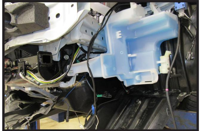
20. Reinstall the windshield washer fluid reservoir attaching it to the frame and baseplate as shown using the existing and provided hardware.
