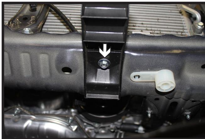
11. Using a 10MM socket, remove the bolt from the belly pan bracket and set aside. Do this on both sides of the vehicle.
