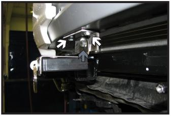
18. **Optional:** Attach the breakaway bracket to the underside of the bumper with two (2) #10-16 x 1" screws (white). Attach the breakaway to the bracket with a 1/4"-20 x 3/4" bolt and 1/4" nut (gray).
