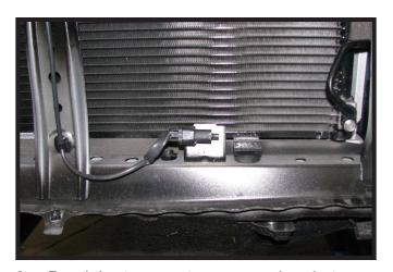
9. Bend the temperature sensor bracket inwards toward the radiator.
