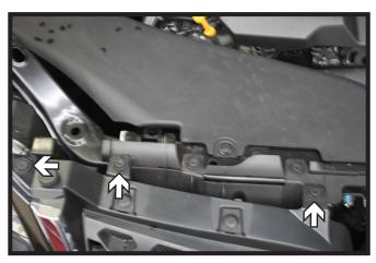
1. Remove the three (3) push pins from the top edge of the fascia. Do this on both sides of the vehicle.
