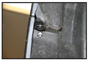
2. In the wheel well where the fascia meets the fender, remove the push pin. Do this on both sides of the vehicle.
