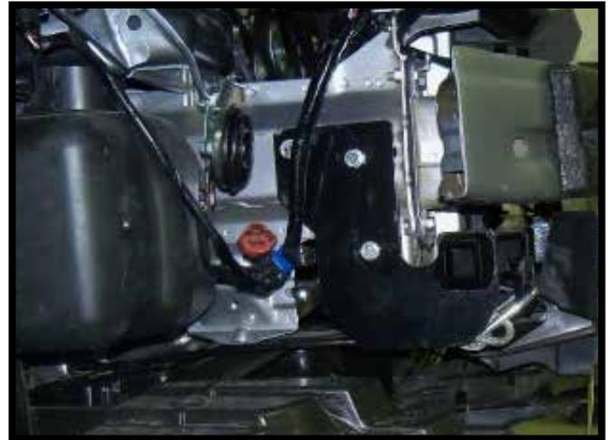
15. Attach the permanent baseplate safety cables to the provided convenience link on the baseplate. Additional options may interfere with suggested mounting; in this case, secure the cables to a solid piece of the frame as described in the instructions included with the permanent baseplate safety cables. Be sure the safety cables do not rub against any hoses or moving parts. Do this on **BOTH** sides of the vehicle.
