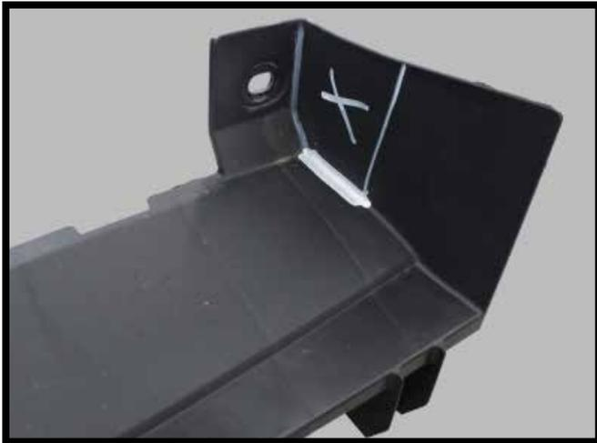
14. Reinstall the air deflector shroud trimming both ends as needed to fit around the baseplate.
