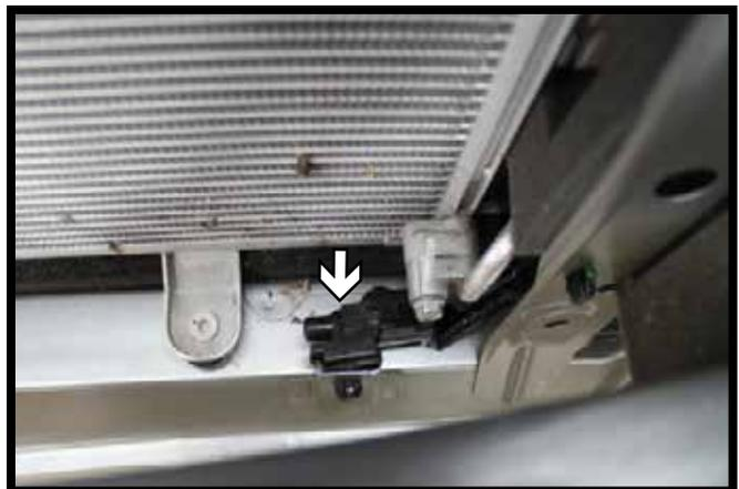
9. Unclip the air temperature sensor from the bracket (left). Relocate the sensor to the backside of the bracket, closer to the radiator to clear the baseplate when installed (right).
