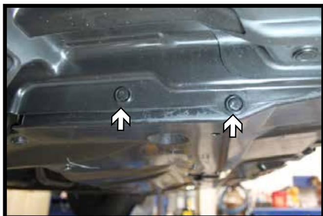
5. Underneath the vehicle on the belly pan, using a flat screwdriver, remove the two (2) push pins from the side of the pan. Do this to both sides of the vehicle.
