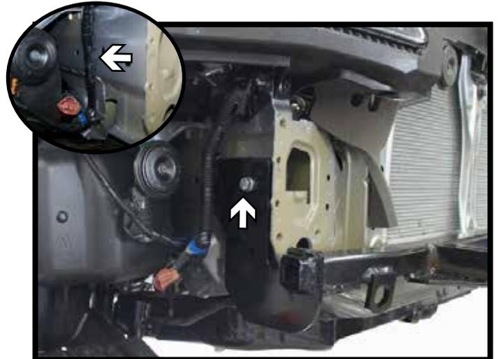
12. Unclip the wire loom from the side of the frame and pull aside. Do this on both sides of the vehicle.
