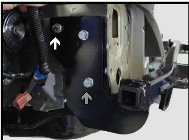
13 Using the holes in the baseplate as a guide, drill the remaining two (2) holes out with a 13/32" bit. Install a 3/8" x 1-1/2" bolt and 3/8" nut into upper hole (white) then a 3/8" x 2" bolt and 3/8" nut into lower hole (gray). Do this on both sides of the vehicle.
