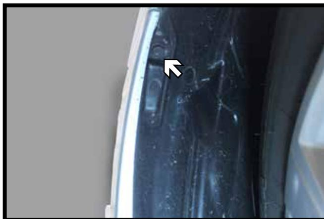
2. Ahead of the front tire, along the upper edge of the wheel well, using a flat screwdriver, remove the push pin. Do this to both sides of the vehicle.
