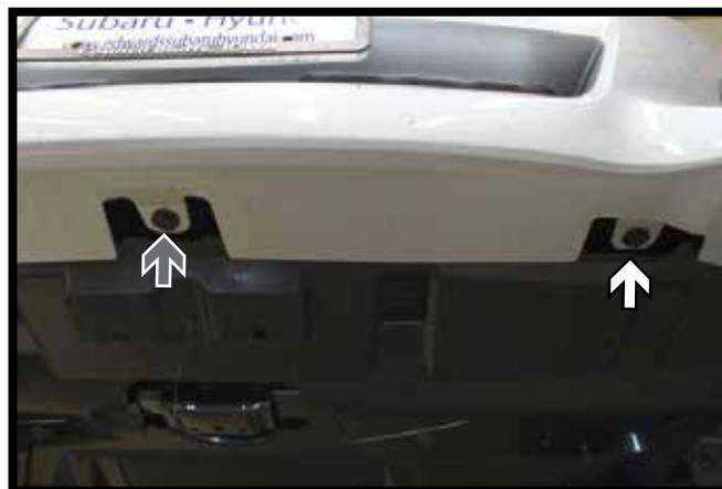
4. Using a flat screwdriver, remove the center push pin (gray) and the two (2) push pins on either side of the center (white). Remove the fascia from the vehicle and set aside.
