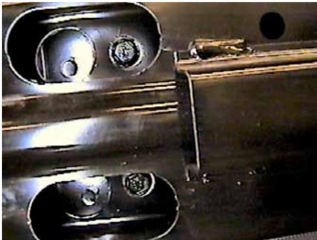
8. Disconnect wire loom and temperature sensor from the top of metal bumper. Remove two metric bolts from metal bumper openings using the 13MM socket, on both sides.
