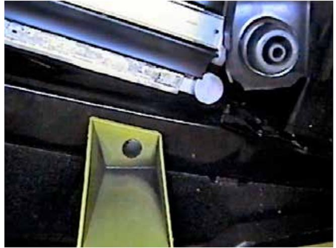
5. Remove the two push pins that attach to the bottom of metal bumper from lower fascia tabs. Pull fascia forward and set aside.
