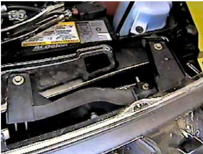
6. Using the 6MM socket, remove two metric bolts from headlight assemblies, pull forward, unplug electrical connections and set aside, on both sides.
