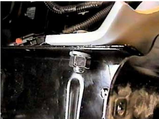
17. Insert hex bolt into the top of baseplate and drilled hole on frame webbing, tighten the 3/8" lock washer and hex nut, on both sides. Be sure to use loctite on all bolts before tightening. Tighten all bolts according to Torque Chart in General Instruction Sheet.
