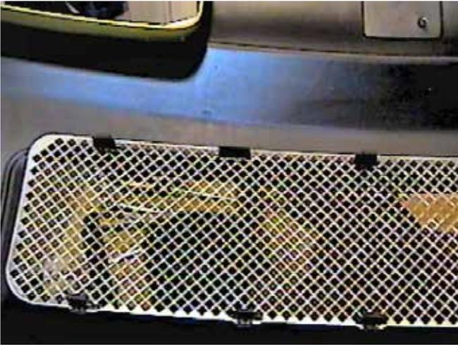
19. Hold fascia to its original position and trim lower mesh grille opening with the diagonal cutters or remove the twelve retainer clips from the back of fascia and completely remove mesh grille. Reinstall fascia.
