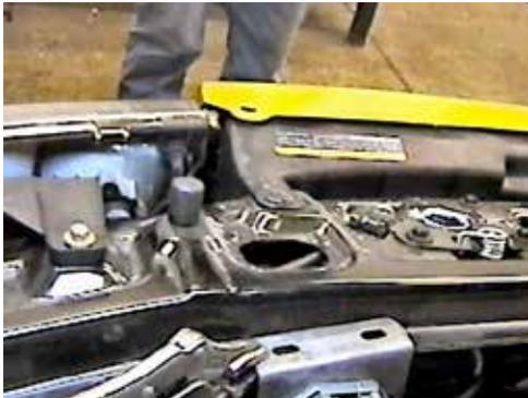
Location for the electrical bracket (101-6135). Clamp with vise grip and drill holes with the 9/32" drill bit.
