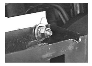
12. Drill a 3/8" hole through the bumper bracket and the frame, use 3/8" hardware as shown in drawing on page 4. Use loctite on all bolts.
