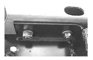
16. Use baseplate as template and drill 3/8" holes. Insert boltplates into bumper placing bolts through the drilled holes. Use appropriate hardware and tighten bolts. Be sure and use loctite on all bolts.
