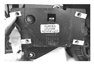
10. Remove the four clips from each bracket. They will not be used in baseplate installation.
