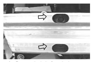
8. Remove the bolts from the bumper exposed by the slots on each side.
