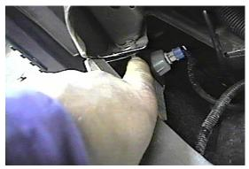
4. There are two 10MM bolt, to remove each side, behind light fixture that hold fascia to fender.
