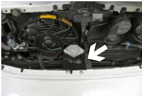
Location for the electrical bracket.
