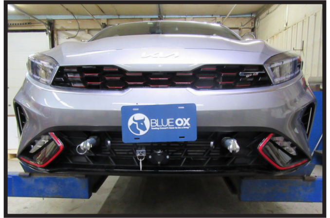
18b. 2022 Models: Hold the fascia as close to its original position, mark and trim the fascia around the convenience links and attachment tabs. Reinstall the belly pan, fascia and reconnect all electrical.
