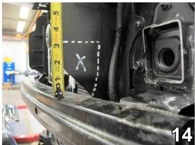
14. Using a utility knife, mark and trim the air dam 3 1/2" up from the metal bumper and horizontally 2 5/8". Do this to both sides of the vehicle, the driver's side is shown.
