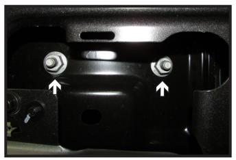
4. Using a 21MM socket, remove the two (2) nuts from the face of the bumper. Do this on both sides of the vehicle.
