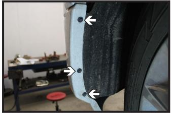
3. Using a 7MM socket, remove the three (3) screws from the edge of the wheel well. Do this on both sides of the vehicle.
