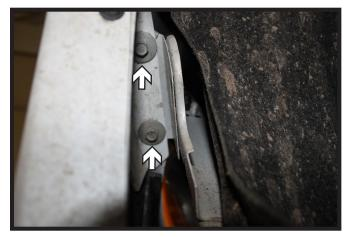
4. Using a 10MM socket, remove the two (2) screws from inside edge of the fascia/ fender joint. Do this on both sides of the vehicle.
