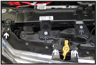
2. Using a T30 Torx, remove the four (4) screws from the top edge of the grille (gray). There are two (2) on each side.
