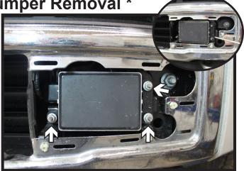
2. If equipped with Adaptive Cruise, using a 11MM socket, remove the three (3) nuts from the ACC sensor. Unsnap the sensor, disconnect the electrical connection and set aside.
