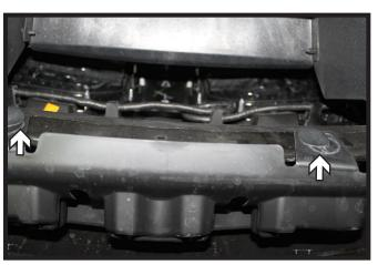
4. On the underside of the fascia towards the middle, remove the two (2) push pins.Pull the corners of the fascia away from
