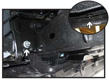
On the backside of the bumper, using a 21MM socket, remove the nut on the outside of the frame. Do this on both sides of the vehicle.
