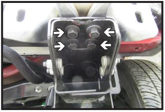
Using an 18MM socket, remove the four(4) bolts from the bottom of the tow hooks on both sides of the vehicle.
