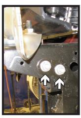
Remove the two (2) bolts from each side of the bracket near the tow hook by using an 18MM socket. Do this on both sides of the vehicle.
