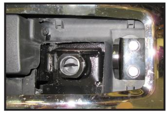
18. Trim the tow hook bolt cover as shown before reinstalling to allow room for the convenience link (left). Do this for both sides of the vehicle. **Note:** For vehicles with ACC, do not reinstall the bolt cover on the driver side of the vehicle (right).
