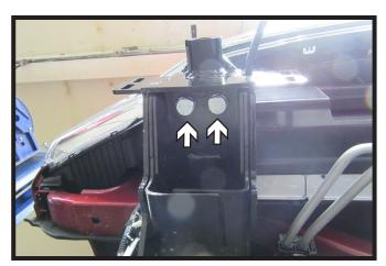
11. Slide the baseplate on, align with the existing front tow hook holes. Bolt on first using two (2) of the 5/8" x 1-3/4" bolts, and lock washers.
