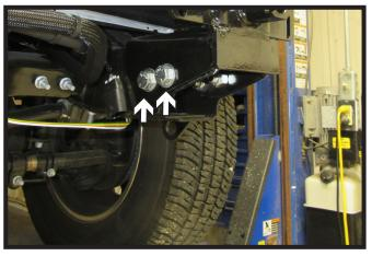
12. Use three (3) 1-3/4" bolts to attach the baseplate towards the outside of the frame. Use a flat washer on the outside and nylon lock nut on the inside for the front two (2) bolts indicated with a white arrows and a flat washer and nylon lock nut on the inside for the third bolt indicated with a gray arrow. Towards the inside of the frame use two (2) 1-3/4" bolts to attache the baseplate with the washer on the outside and nylon lock nut on the inside. Do this on both sides of the vehicle.
