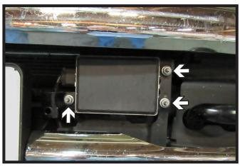
5. **Models with ACC:** Using an 11MM socket, remove the three (3) bolts holding the ACC onto the driver side of the vehicle. Unplug, remove, and set aside the ACC to be reinstalled later.
