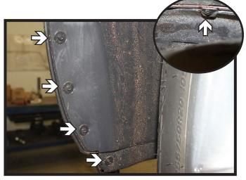
2. Using a 5.5MM socket, remove the seven (7) screws from the edge of the wheel well. Then above the center of the wheel, remove the push pin (inset). Do this on both sides of the vehicle.
