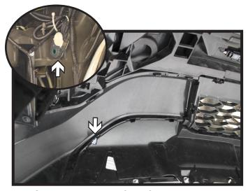
15. On the backside of the fascia trim the outer tab shown flush with the backside of the fascia for clearance of the baseplate.
