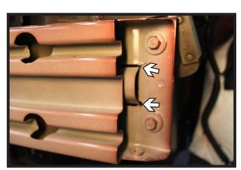
9. At the end of the bumper, using a reciprocating saw, trim off the rib in both places as shown for nut plate access. Do this on both sides of the vehicle.
