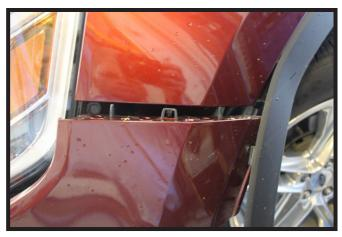
5. Lift up on the corners of the fascia to unsnap and pull it away from the vehicle disconnecting any electrical connections and fluid lines. Set the fascia aside.
