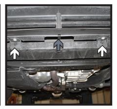
8. **Shutter Models Only:** On the driver side, remove the two (2) screws from the shutter motor and unsnap from the housing (left).
