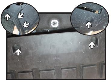
Using a 7MM socket, remove the eight
