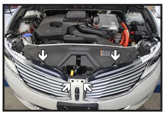
1. Using a T25 Torx, remove the four (4) screws from the top edge of the fascia.
