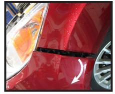
4. On the underside of the fascia, remove the two (2) push pins from the center (left). Then remove the four (4) remaining push pins, two (2) on either side of the center push pins (middle). Pull the corners of the fascia out and forward to unclip and remove from the vehicle (right).
