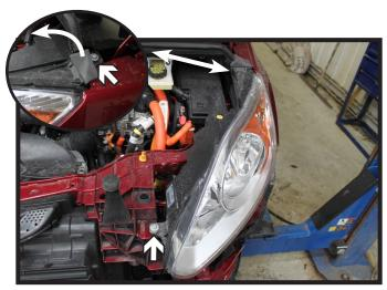
8. Using a T27 Torx, remove the two (2) screws from the front and back of the headlight. Lift up on the rear of headlight to release and unhook the wiring. Set the headlight aside. Do this on both sides of the vehicle.
