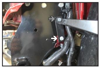
13. On the driver side, install the attachment plate to the existing tab, using the existing bolt (white). Bend the tab back to it's original position, then connect the air box to the attachment plate with a 1/4"-20 x 3/4" bolt and 1/4" nylon nut (gray). Secure any loose wiring.
