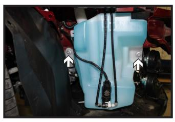
5. On the passenger side, using a 10MM socket, remove the two (2) screws from the washer fluid reservoir. Disconnect lines and set reservoir aside.
