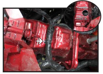
Behind the headlights, unclip the wiring loom to expose the existing hole. Using a 1-1/4" hole saw, drill the existing hole for access to install the baseplate nut plate. Do this on both sides of the vehicle.
