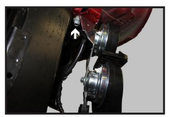
Using a 10MM socket, remove the screw from the backside of the horn bracket and set the horn assembly aside.
