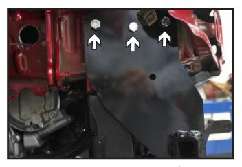
11. Using the existing holes in the frame, bolt the baseplate to the vehicle with the 3/8"-16 x 1-1/2" bolts and 3/8" nut plates. Ream out the holes if necessary for bolt clearance. Do this on both sides of the vehicle. Make sure baseplate is level before tightening down fasteners.
