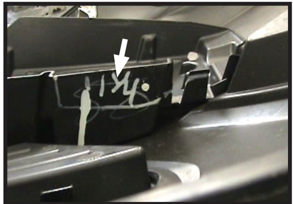
21. Measure down 1-1/4" and all the way over to the outer edge on the backside of the front fascia. Notch this as shown to allow for proper clearance.
