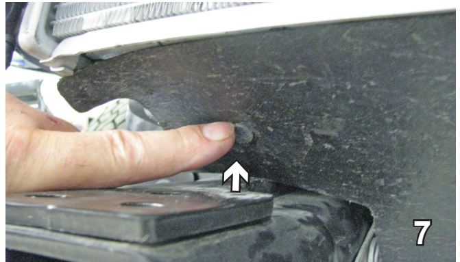
7. On the passenger side, on the back bottom of the lower radiator, remove the push pin from the rubber air dam. Set the pin and the air dam aside to be reinstalled later.
