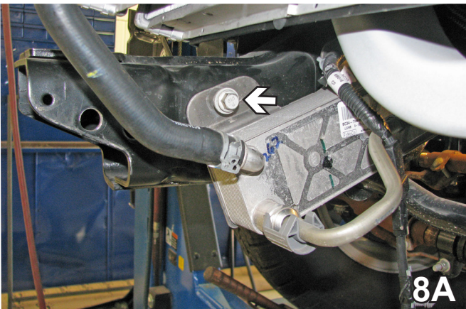
8. Using a 13MM socket remove the three metric bolts from the coolant transfer box on the passenger side to be reinstalled later. Pull the box out of the way so that the side holes can be drilled in step 12 using the baseplate as a template.
