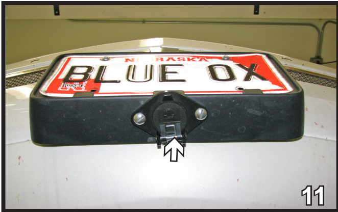
11. Attach the electrical bracket under the license plate.
