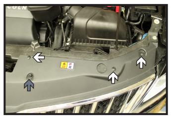
Remove the three (3) push pins (white) and then, using a 10MM socket, remove the one (1) screw (gray) from the plastic radiator cover. Do this to both sides of the vehicle.
