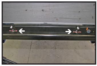
Using a reciprocating saw, cut off the tabs that the lower coolant line were attached to, being careful not to cut into the radiator.
