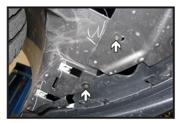
Using a 5.5MM socket, remove the two (2) screws from underneath the front edge of fascia. Do this to both sides of the vehicle.
