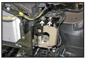
12. Place baseplate on top of frame and line up the holes in the baseplate with the two (2) existing holes on top of the frame. Reinstall the four (4) existing bolts from step 6, two (2) on the top (white) and (2) on the face (gray). Do this to both sides of the vehicle.
