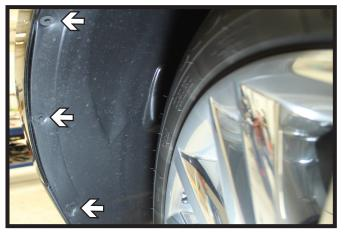
Using a 5.5MM socket, remove the three
