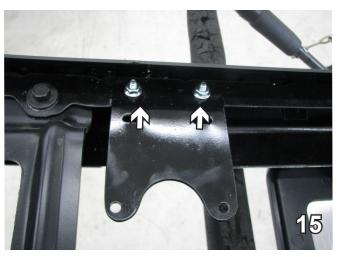
15. Install 1/4-20 x 3/4" bolts with 1/4" flat washers, 1/4 lock washers and 1/4-20 whiz nuts.
