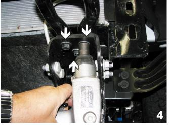
4. Remove the tow hook by removing the three bolts underneath it using a 15MM socket. Set tow hooks and bolts aside--they will not be used again. Use a 17/32" drill bit to ream the two front holes. Do this on both sides.
