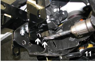
11. Align the baseplate with the existing holes in the frame, With the baseplate as a template, use a 17/32" drill bit to ream out the holes on both sides of the frame rail if needed. Do this on both sides of the vehicle.
