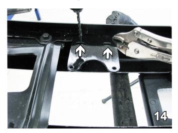
14. Place the metal bumper face down. Position the electrical bracket over the two existing holes on the inside top driver's side. Drill out the hole on the left using a 5/16" drill bit.
