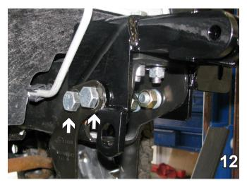
12. Slide the lower support bumper brace back over. It may need to be widened a bit.
