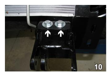
10. Slide the baseplate over the frame rail. Align with the top holes. Insert 1/2-13 x 3 1/2" hex bolts with 1/2" flat washer on the top. Attached to 1/2" lock washers and 1/2-13 hex nuts. Do this on both sides. Tighten with Loctite Red.
