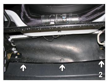
2. Remove three push pins from the bottom edge of the plastic cover. Set cover and push pins aside to be reinstalled later.
