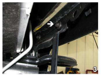
Remove the bolt which is exposed after removal of the cover. Set the bolt aside to be reinstalled later.
