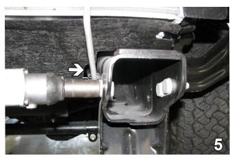
On the driver's side, it will be necessary to pull the Christmas tree pin from the coolant line bracket that goes into the frame in order to position the baseplate. It will be reinstalled later.
