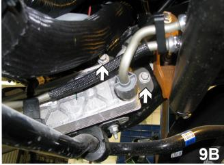
9. Using a 13MM socket remove the three metric bolts from the coolant transfer box on the passenger side. Then pull the box out of the way so that the side holes can be drilled using the baseplate as a template.
