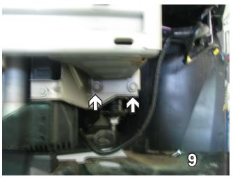
Using the 13MM socket, remove two bolts from underneath the bumper. Do this to both sides. Set the bolts aside to be reinstalled later.
