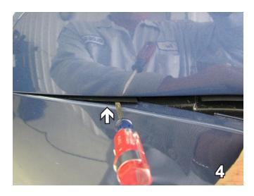
4. Grab, lift and pull the fascia straight out to remove it. When you come to the tabs, use a screwdriver to lift up and pop the fascia out. Do this to both sides of the vehicle. Set fascia aside carefully to be reinstalled later.
