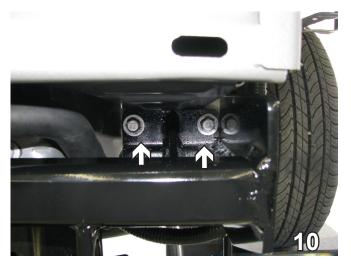
10. Slide the baseplate up into place, start the two existing bolts. Do this to both sides of the vehicle.
