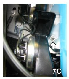
7. On the passenger side using the 10mm socket, remove three metric bolts from the washer reservoir, one on the right side (see 7A) and two on the left (see 7B & 7C). Disconnect the hoses and the wiring, plug the hoses. Set washer reservoir and bolts aside to be reinstalled later.
