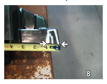
8. On the bottom side of the plastic bumper cover, using a utility knife, notch out the corner. Go over 1", then up, across and back. Do this to both sides.
