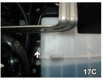
17. Using the utility knife, cut the tab off of the washer reservoir. Reinstall the washer reservoir. Use 6MM-1 x 45MM hex bolts with 6MM lock washers and 1/4" flat washers. Insert 1" spacers between the washer reservoir and the frame for each hole. Reconnect the hoses and the wiring. Reinstall the plastic bumper cover. Tighten all bolts completely.
