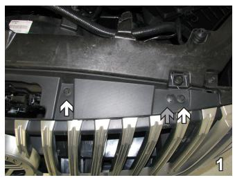
Using the 10mm socket, remove two metric bolts from the top of the grille (white arrows). Remove one pushpin from the top of the grille (gray arrow). Do this to both sides of the vehicle. Set bolts and pushpin aside to be reinstalled later.
