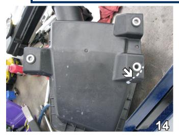
14. On the driver side, trim the corner of the air baffle up to the rubber as shown.
