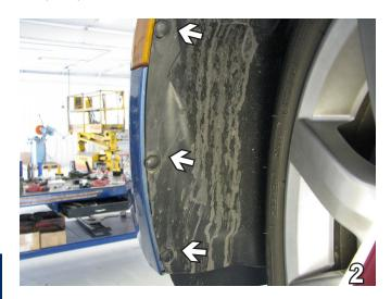
Just forward of the front tire, inside the wheel well, remove three pushpins. Do this to both sides of the vehicle. Set pushpins aside to be reinstalled later.
