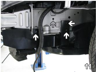
11. On the driver side, the plate is bent. You may need to pull it out a little to get by the ridge. Be sure the baseplate is level with respect to the vehicle frame. Using the baseplate as a template with the 13/32" drill bit, drill the three holes on the side (white arrows). Using the 1 1/4" hole saw, drill a hole so that nut plates may be inserted into the frame (gray arrow). Do this to both sides of the vehicle.
