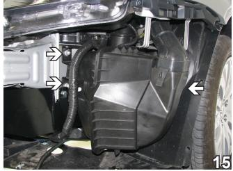
15. Reattach the air baffle.
