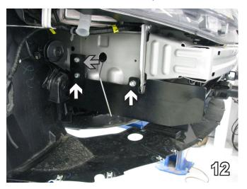
12. On the passenger side, insert 3/8-16 x 2" hex bolts in all holes, 1" spacer tubes are placed between the baseplate and the frame for each hole. The front hole and the bottom back hole have 3/8" lock washers with 3/8-16 hex nuts (white arrows). The top back hole has the 3/8" lock washer on this side and a 3/8-16 nut plate inserted into the drilled hole (gray arrow). Be sure to use Loctite on all the bolts.
