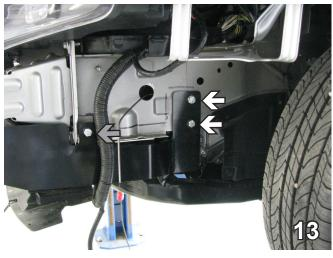
13. On the driver side, insert 3/8-16 x 2" hex bolt in the front hole (gray arrow), a 1" spacer tube is placed between the baseplate and the frame, 3/8" lock washer with 3/8-16 hex nut. The back holes (white arrows) have 3/8-16 x 1 1/2" hex bolts. The bottom back hole has 3/8" lock washer with 3/8-16 hex nut. The top back hole has the 3/8" lock washer on this side and a 3/8-16 nut plate inserted into the drilled hole. Be sure to use Loctite on all the bolts.
