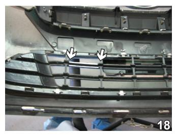
18. Using the utility knife, on the back side of the fascia, cut out the first long top rib. Do this to both sides of the fascia. Reinstall the fascia.
