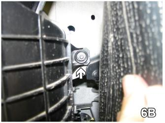
6. On the driver side use the 13MM socket to remove the three metric bolts from the air baffle, two in the front and one in the back. Set the bolts and air baffle aside to be reinstalled later.
