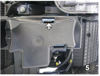
Remove the plastic bumper cover by pushing down on the eight tabs across the top to release. Set the bumper cover aside to be reinstalled later.
