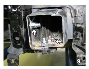
9. View of the frame end, showing all the bolts installed.
