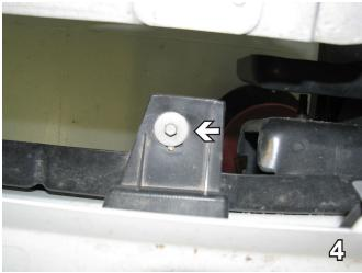
Using the 8MM socket, remove three bolts just behind the fascia across the front. Remove the fascia and set aside.
