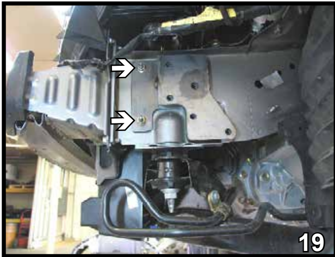
19. On the driver's side frame rail, align the spacer plate with the existing air baffle studs. Install the 3/8" flat washers and existing air baffle hex nuts to the air baffle studs and tighten. Note: Actual spacer plates will be painted powder-coat black.
