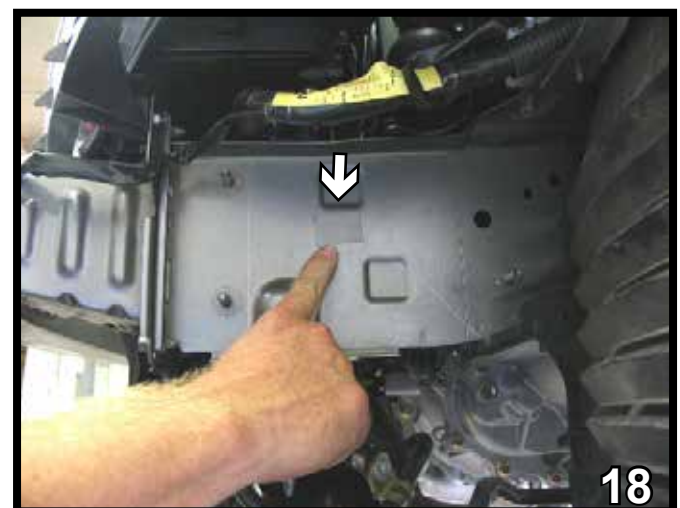
18. On the driver's side, remove a piece of tape from the center of the frame rail. Do this to both sides of the vehicle.
