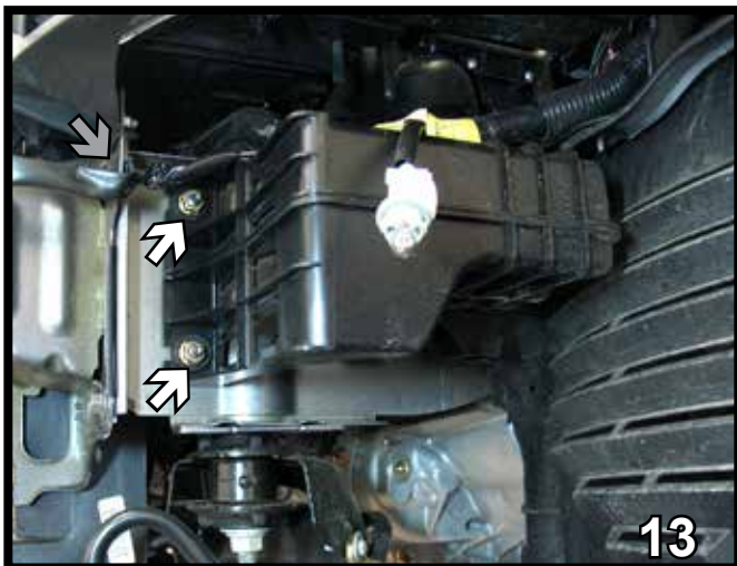
13. On the driver's side, remove two metric bolts from the left side of air baffle using the 13mm socket (see white arrows). On the upper right corner of bumper bracket (see grey arrow), squeeze clips together to release wiring. Move wiring out of the way. Set bolts aside to be reinstalled later.
