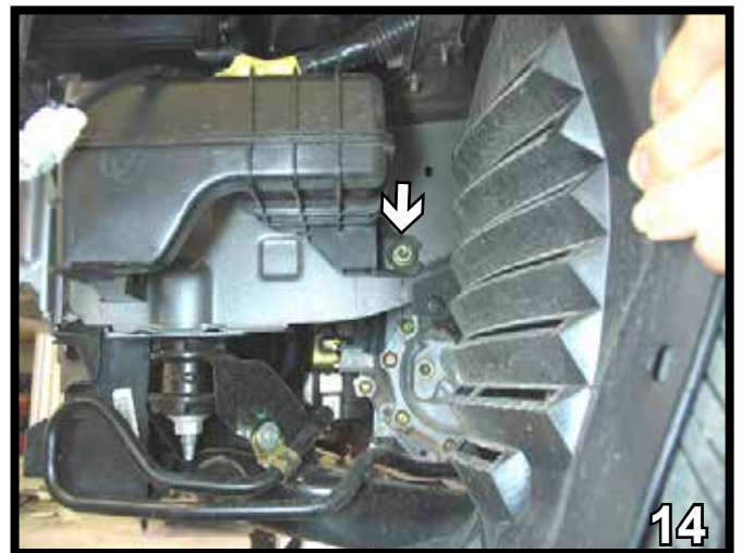
14. Using the 13mm socket, remove one metric bolt from the lower right corner of air baffle. Slide air baffle down and away from its upper tubing to remove. Two rubber bushings from left side of air baffle will not be reinstalled. Set bolt and air baffle aside to be reinstalled later.
