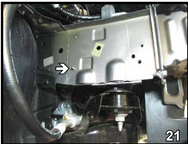
21. On the lower left of passenger's side frame rail, use the vice grips to break off the washer reservoir stud.
