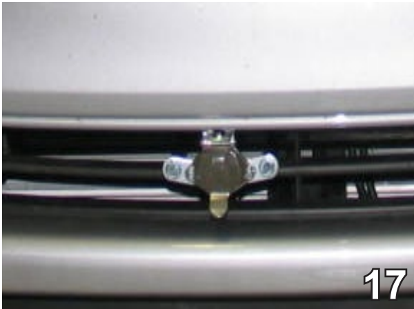
17. Location for the 4 or 6 pin electrical coupler on the fascia's lower air dam just below license plate.
