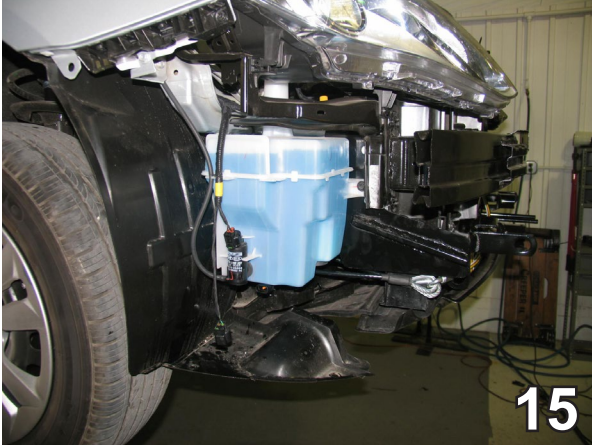
15. Reinstall the washer reservoir on the passenger side, using the existing bolts. Be sure that all the electrical connections and hoses are plugged in properly.
